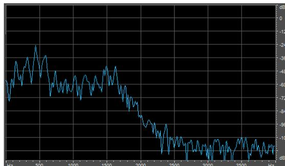
(b) FFT of Low-pass Filtered Signal
