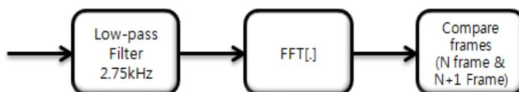
**Figure. 2.** General Signal Processing in Speech Signal.
