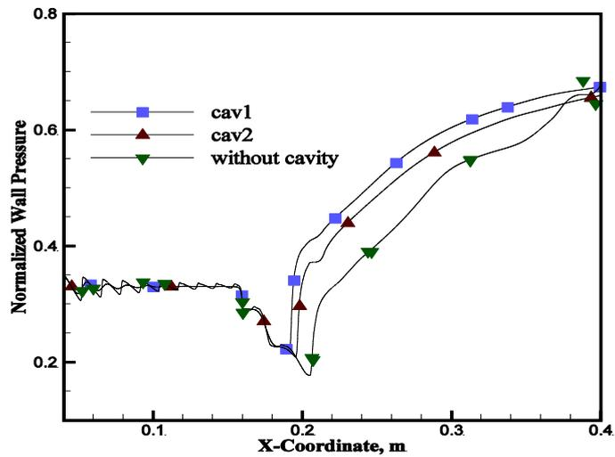
**Figure. 6.** Distribution of pressure normalized for cases with holes and without a cavity wall
