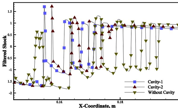
Figure. 8. Distribution function of  $\frac{u}{a} \frac{\nabla P}{\sqrt{P_x^2 + P_y^2 + P_z^2}}$  the central line conduit for cases with
