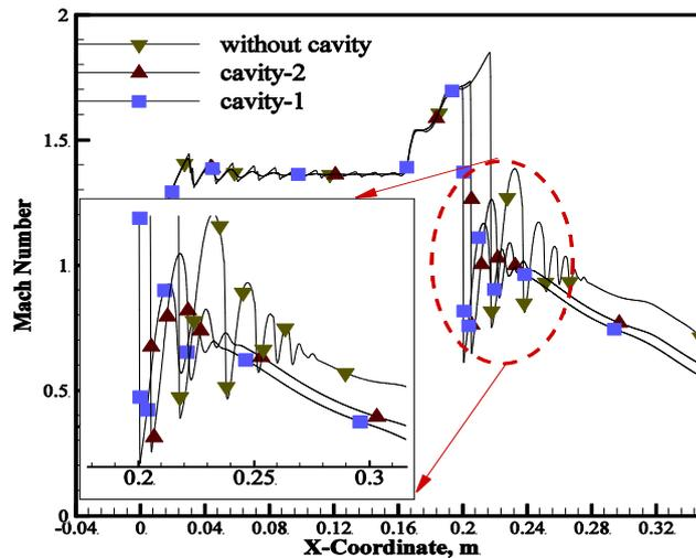
**Figure. 7.** Distribution of Mach number on the center line conduit for cases with The cavity And the without The cavity
