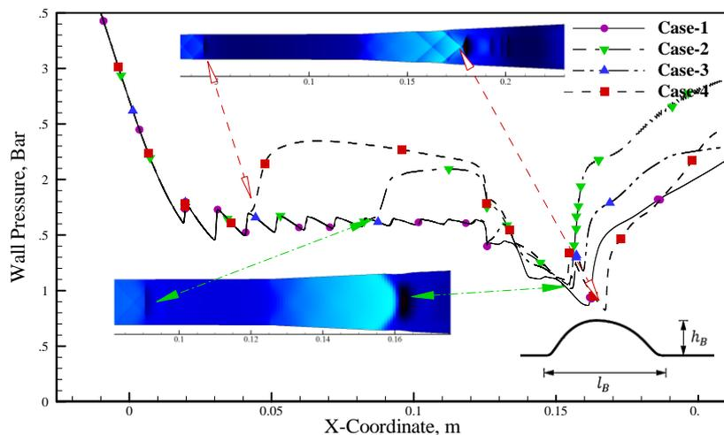
Figure. 4. Distribution of pressure walls with lumps and without that
