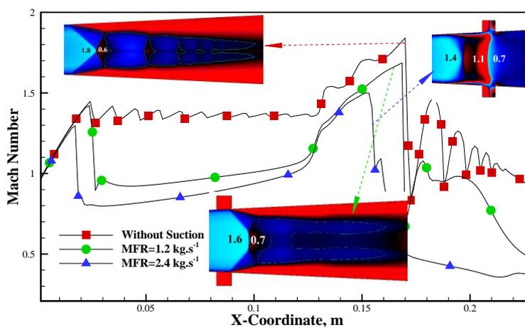
**Figure. 9.** Distribution of Mach number on the center line of the duct
