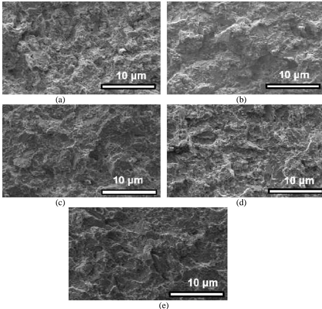
**Figure. 8.** SEM micrographs of fractured surfaces of Ti64 powders sintered at 850 °C and held for: (a) 2 min, (b) 4 min, (c) 6 min, (d) 8 min and (e) 10 min.
