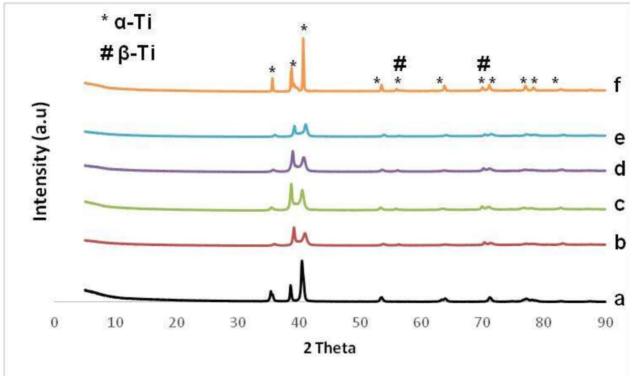
**Figure. 5.** XRD pattern of (a) as-received Ti64 powder and Ti64 alloys sintered at 850 °C and different holding times (b) 2 min, (c) 4 min, (d) 6 min, (e) 8 min and (f) 10 min.
