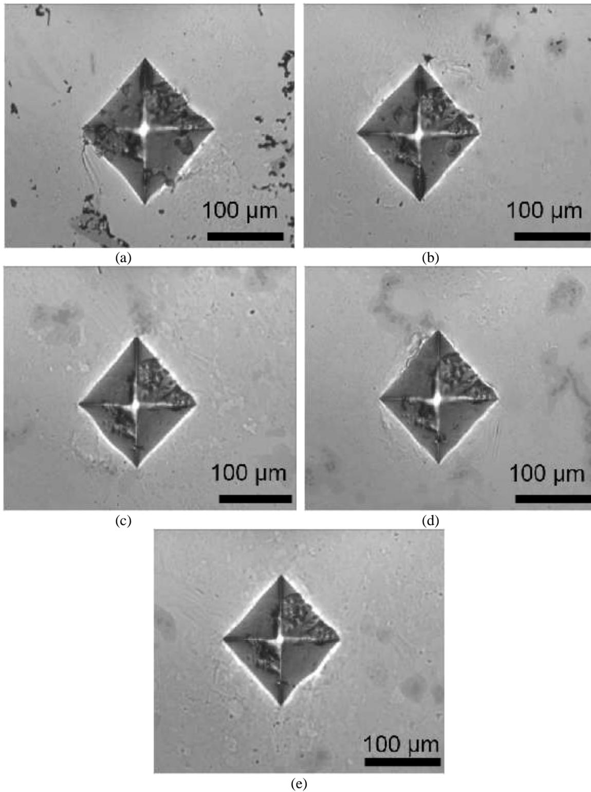
**Figure. 7.** Microhardness indentation micrographs for Ti64 alloys held for: (a) 2 min, (b) 4 min, (c) 6 min, (d) 8 min and (e) 10 min respectively at 850 °C sintering temperature
