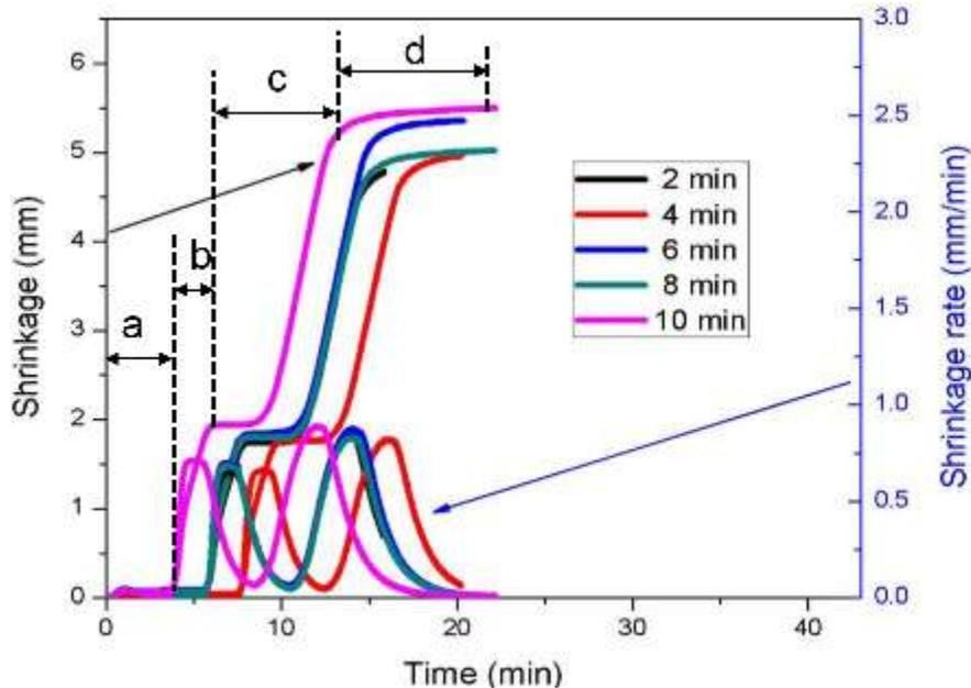
**Figure. 2.** Retrieved sintering profile of sintered samples at different holding times.
