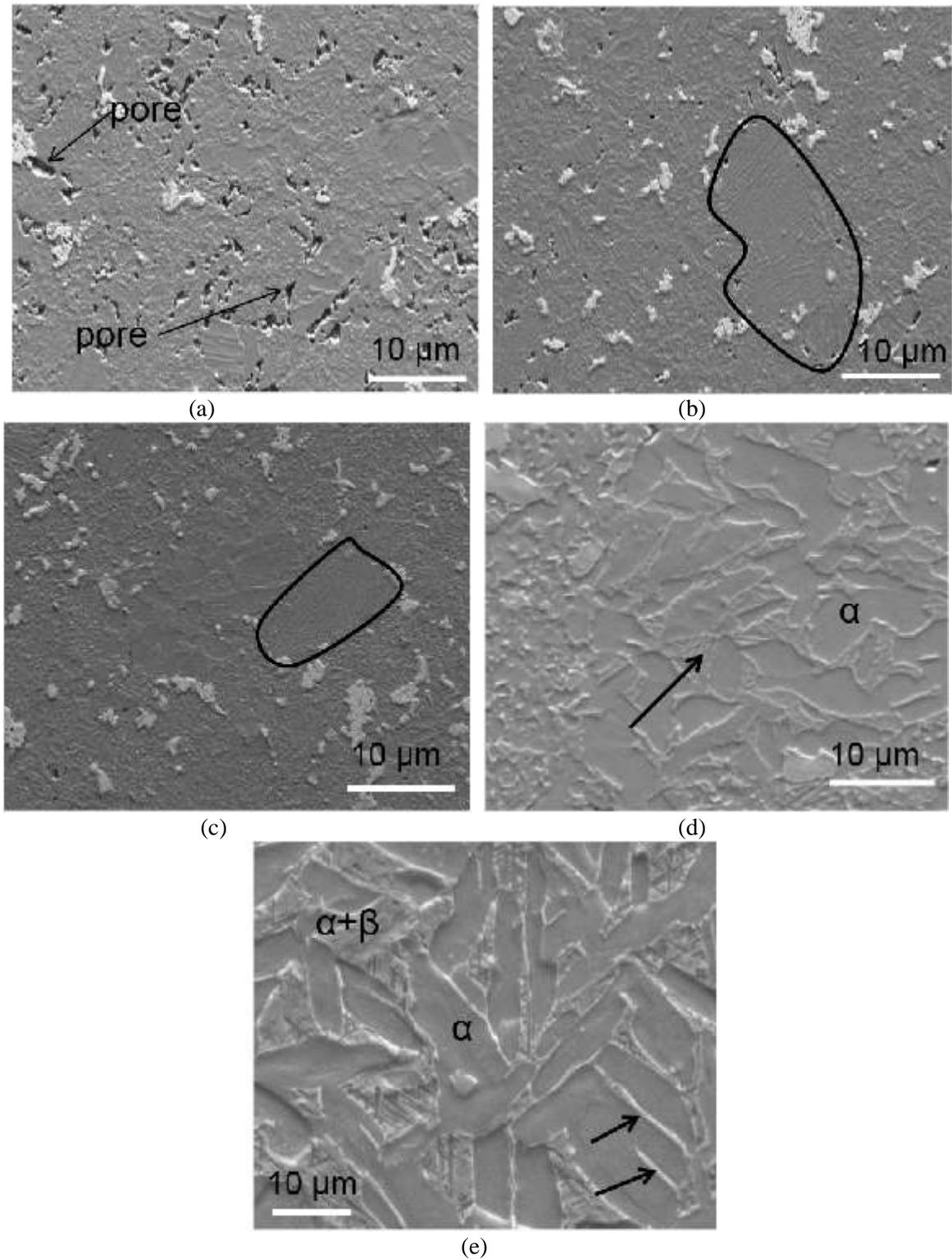
**Figure. 4.** SEM micrographs of Ti64 powders sintered at varied holding times (a) 2 min (b) 4 min (c) 6 min (d) 8 min (e) 10 min.
