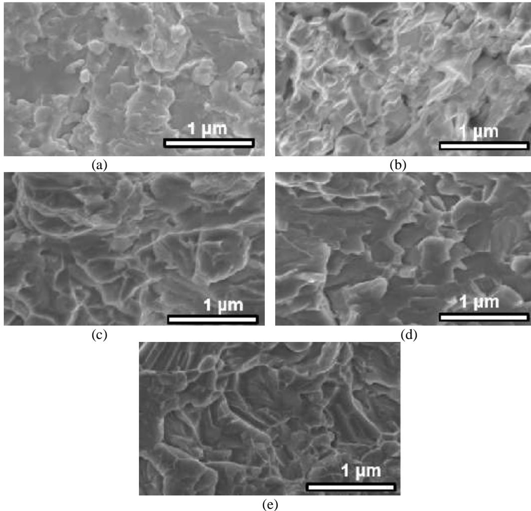
**Figure. 9.** Corresponding high magnification SEM micrographs for fractured surfaces of Ti64 powders sintered at 850 °C and held for: (a) 2 min, (b) 4 min, (c) 6 min, (d) 8 min and (e) 10 min respectively.
