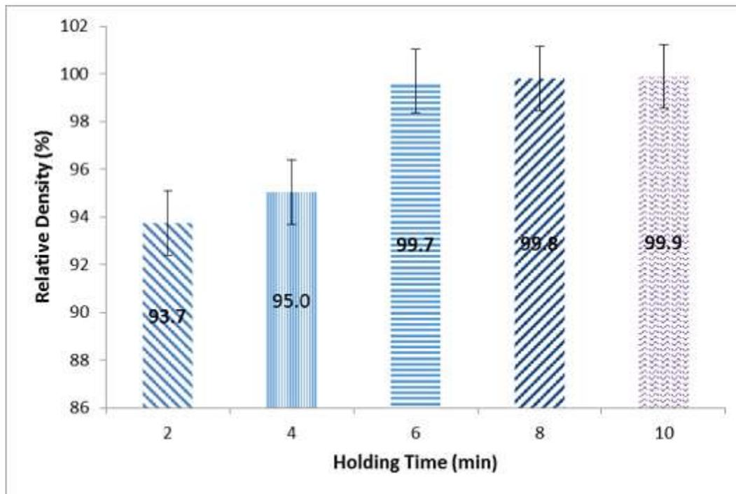
**Figure. 3.** Relative densities of sintered samples at different holding times.
