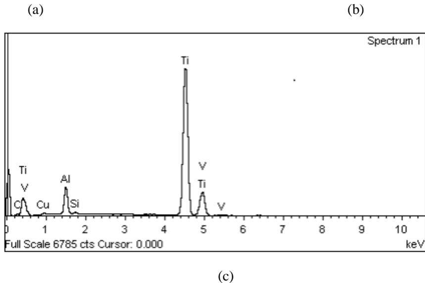
**Figure. 1.** SEM micrographs of as-received Ti64 powders at (a) low and (b) high magnifications, with corresponding (c) EDS spot analysis.
