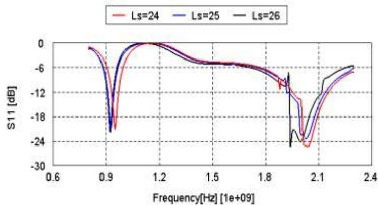
Figure.3. Simulated  $S_{11}$  versus frequency by varying the parameter  $L_s$
