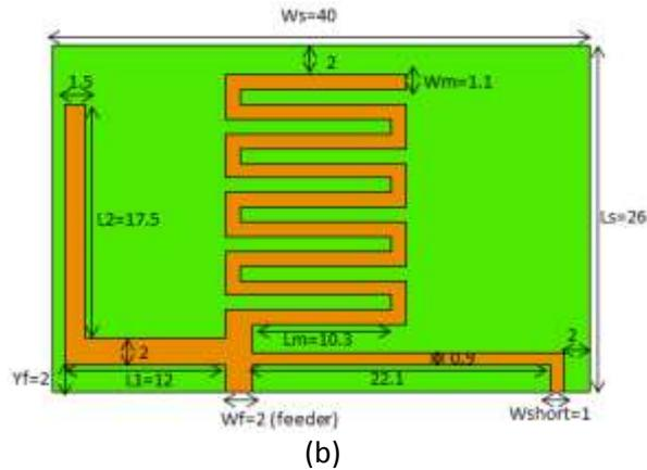
Figure. 1. (a) 3-D geometry of the proposed antenna. (b) Patch antenna geometry as seen from above in mm
