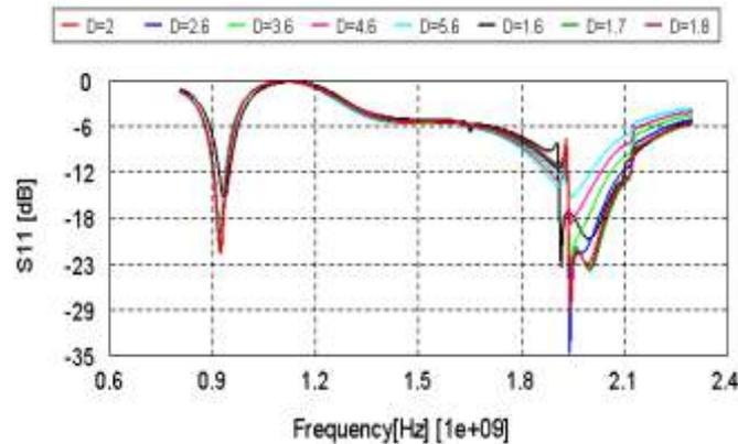
Figure.4. Simulated S11 versus frequency by varying the height D in mm
