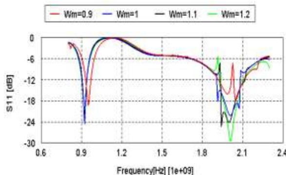
Figure.6. Simulated S11 versus frequency by varying the parameter  $W_m$
