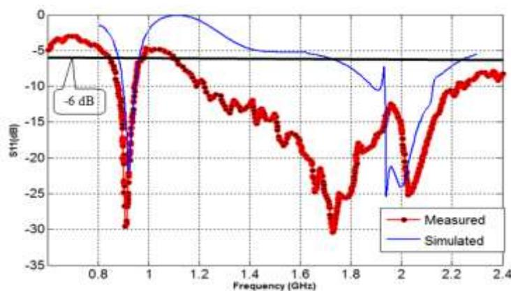
Figure.10. Simulated and measured S11 versus frequency of the realized antenna
