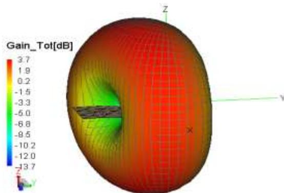
Figure.13.The 3D total gain pattern of miniaturized antenna at  $f_2=1.908$  GHz
