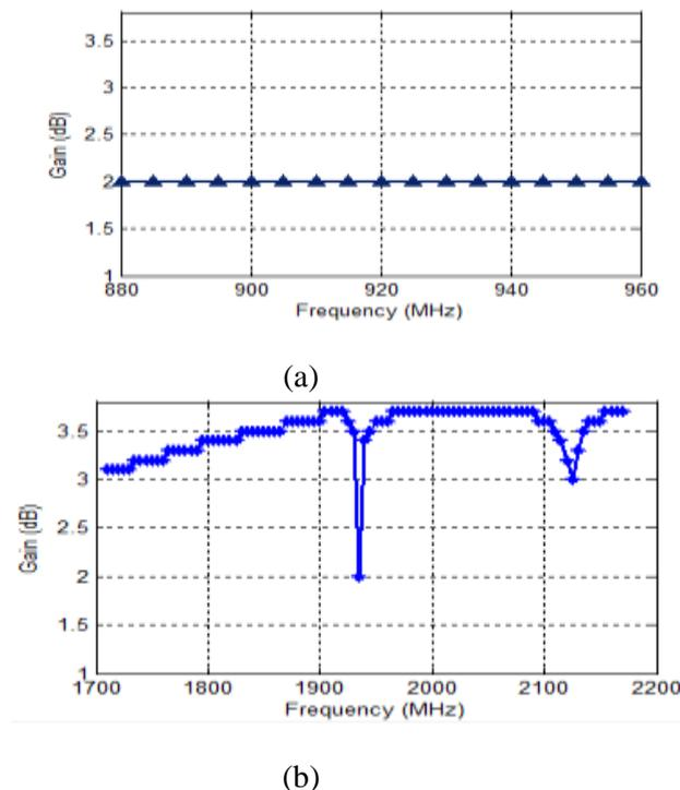
Figure.11. Maximum gain of the proposed antenna: (a) GSM900 band, (b) GSM1800, PCS and UMTS bands
