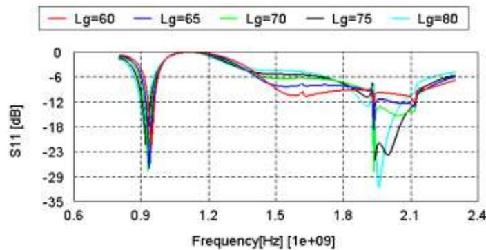
Figure.8. Simulated  $S_{11}$  versus frequency by varying the parameter  $L_g$
