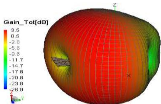
Figure.14.The 3D total gain pattern of miniaturized antenna at  $f_3=1.944$  GHz
