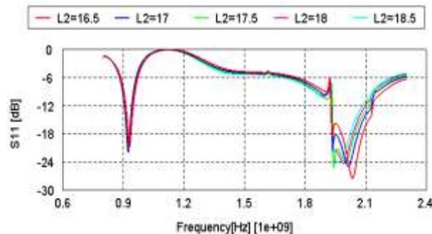
Figure.7. Simulated S11 versus frequency by varying the parameter L2
