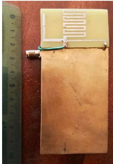
Figure.9.The Realized Antenna
