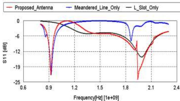
Figure. 2. Simulated reflection coefficients for the proposed antenna, the meandered line radiator, and the L-shaped radiator
