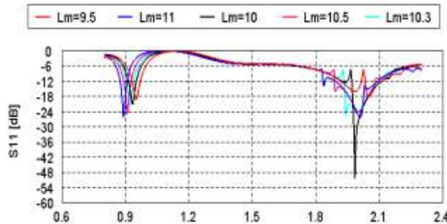
Figure.5. Simulated S11 versus frequency by varying the parameter  $L_m$
