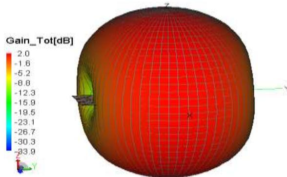
Figure.12.The 3D total gain pattern of miniaturized antenna at  $f_1=0.92$  GHz
