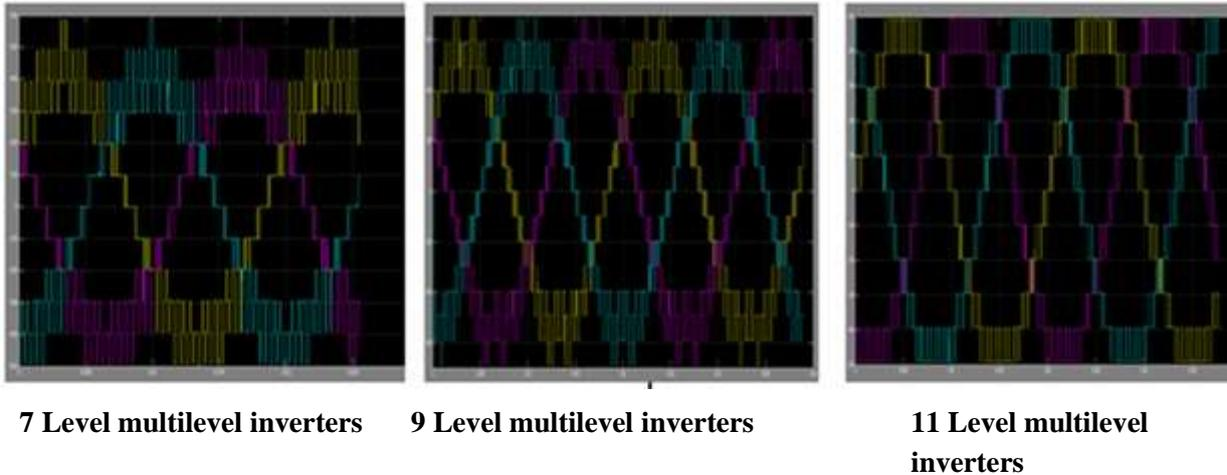
**Figure 4: Output phase voltage waveforms for various level numbers**
