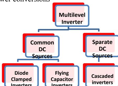
**Figure 2:** Classification of multilevel inverters
