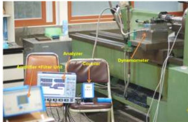
**Fig.5** Experimental set-up for finding modal data
