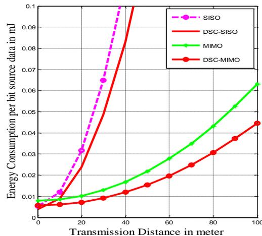
**Figure.6.** The energy consumption per bit of DSC-MIMO, CMIMO, DSC-SISO and SISO at constellation size  $b=4$  bits /symbol
