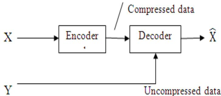
**Figure.1.** Data compression using Distributed source coding
