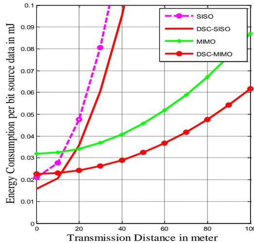
**Figure.4** The energy consumption per bit of DSC-MIMO, CMIMO, DSC-SISO and SISO at constellation size  $b=1$  bit /symbol
