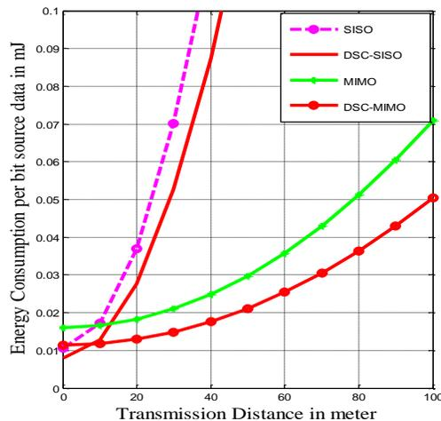
**Figure.5** The energy consumption per bit of DSC-MIMO, CMIMO, DSC-SISO and SISO at constellation size  $b=2$  bits /symbol
