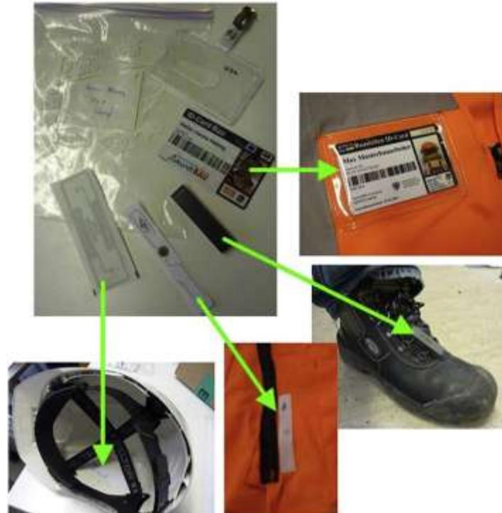
Fig. 2 RFID tag on personal protective equipment [32]
