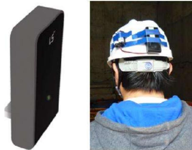
Fig. 11 Safety helmet with RFID tag [5]
