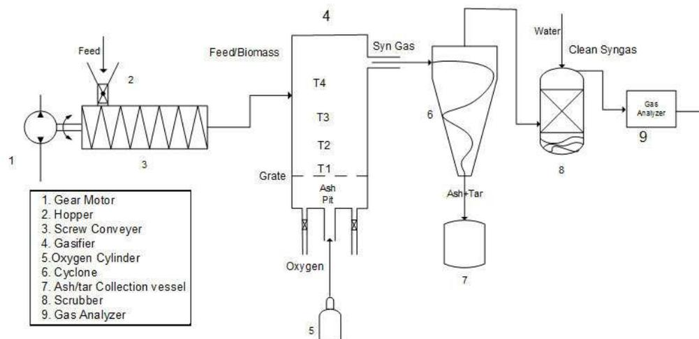
Figure 1 Flow diagram for Gasification Process
