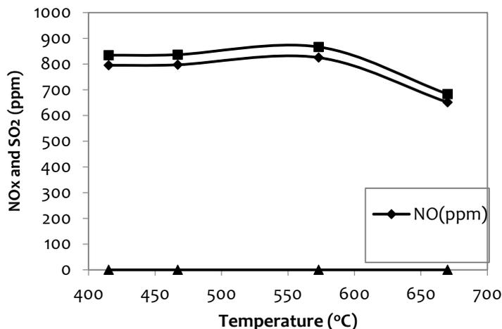
Figure 4 Temperature Effect on NO<sub>x</sub> and SO<sub>x</sub> for (a) without circulation (b) with circulation
