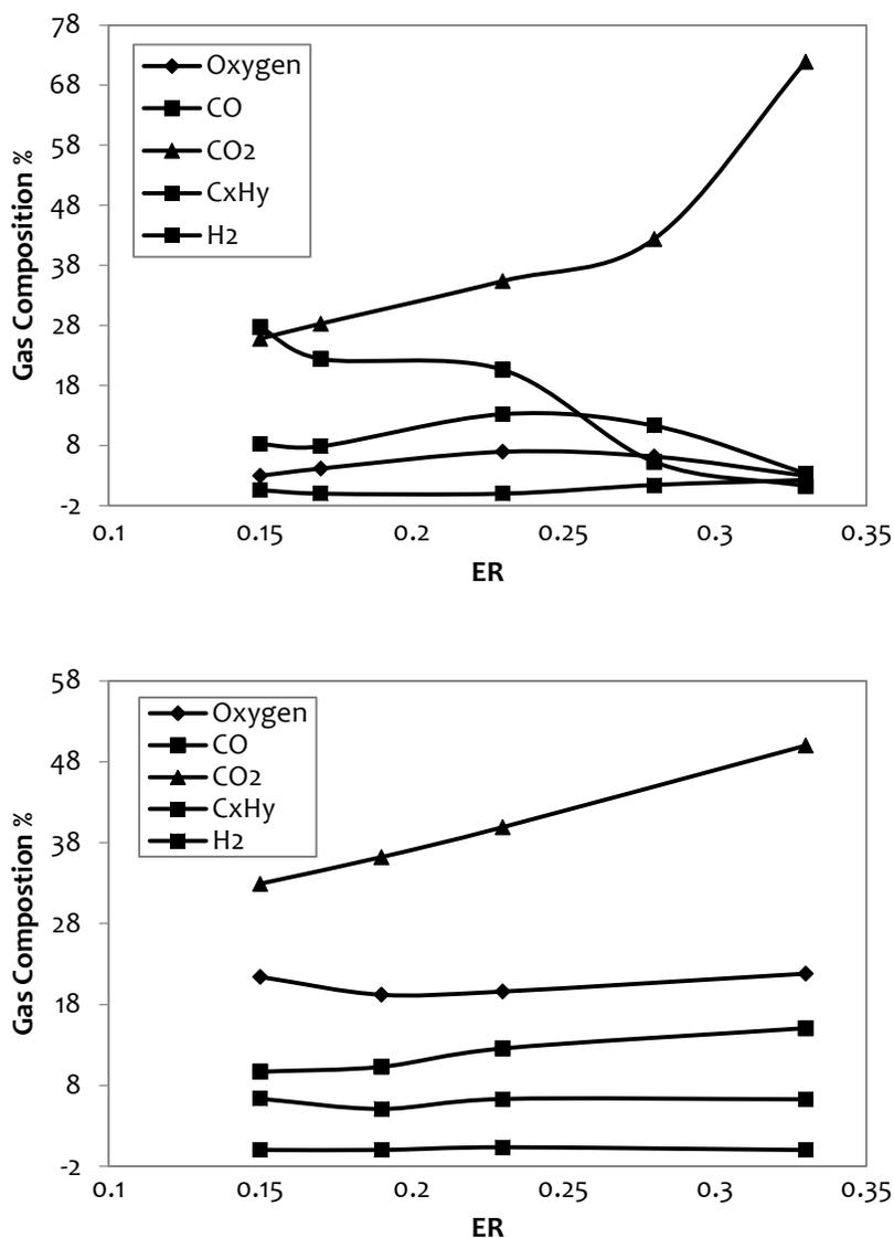
Figure 6. ER Effect on Gas Composition (%) for (a) without circulation (b) with circulation
