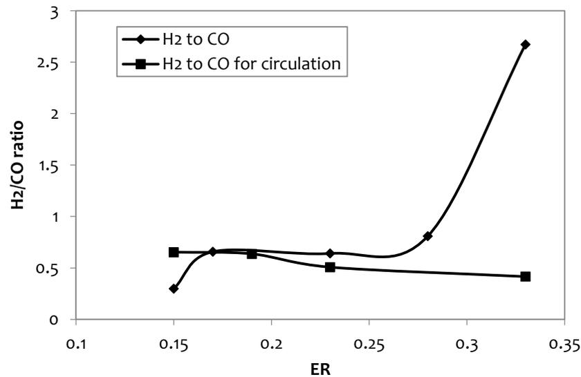
Figure 8 ER Effect on H<sub>2</sub>/CO ratio
