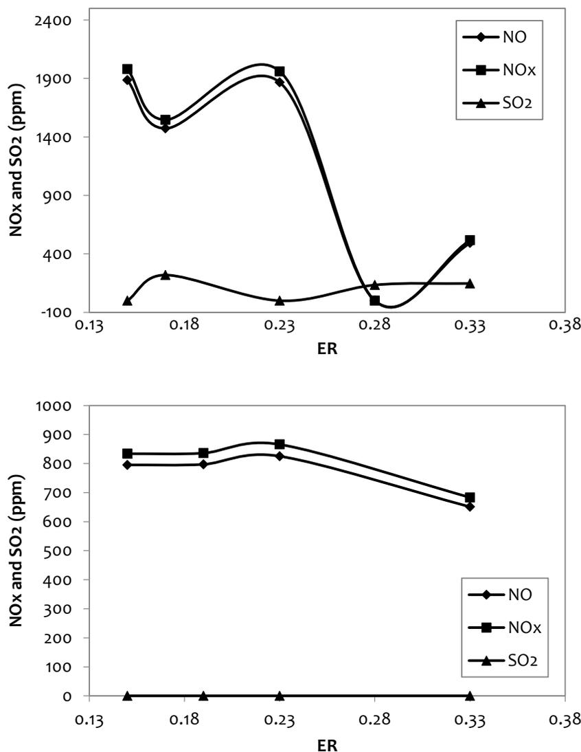
Figure 7 ER Effect on NO<sub>x</sub> and SO<sub>2</sub> formation for (a) without circulation (b) with circulation
