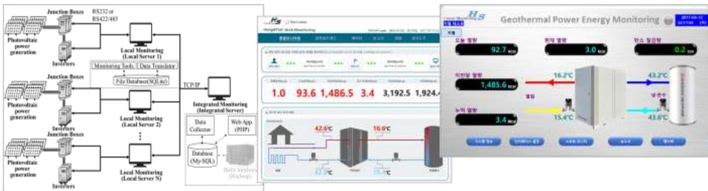
Fig. 10. The target program of an integrated Solar & Geothermal power energy monitoring system
