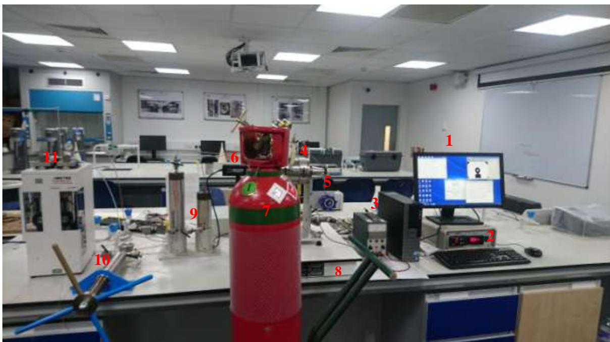
**Fig. 2:** Experimental set-up for IFT measurement (1-Data acquisition system; 2-Temperature and pressure recorder; 3-Illuminator; 4-IFT Measurement Chamber; 5-Back-pressure regulator; 6-Rame-hart Camera; 7-Methane cylinder; 8-Vibration control table; 9-water sample cylinder; 10-Manual pump; 11-Automatic pump)
