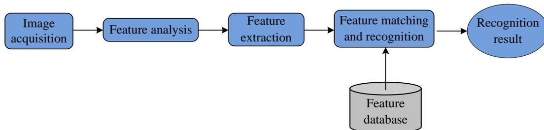
Figure 1. Texture target recognition system
