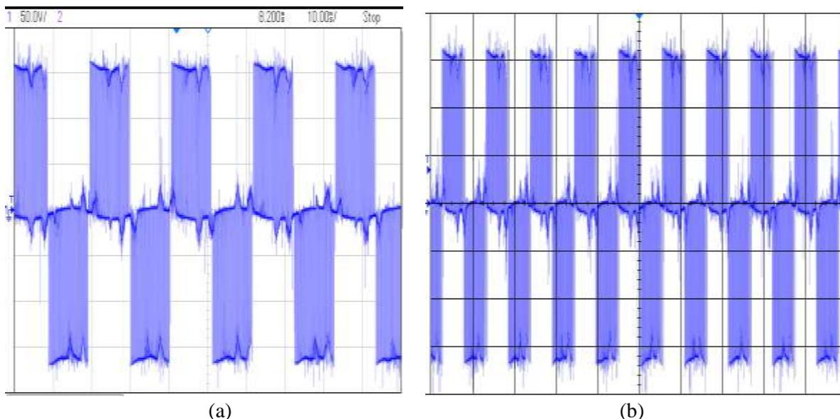
Fig.26. Common mode voltage (a) a-phase (b) b-phase
