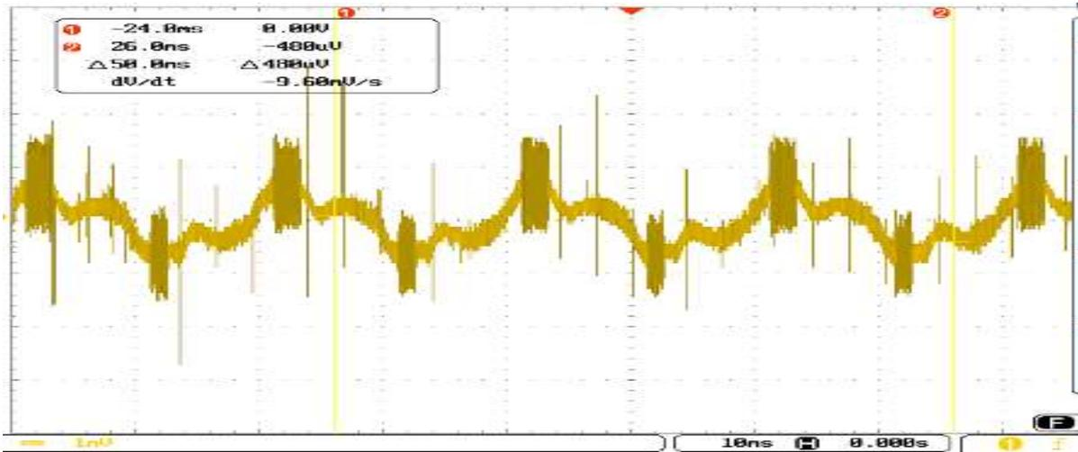
Fig.24. Input current of matrix converter with 3-phase IM drive
