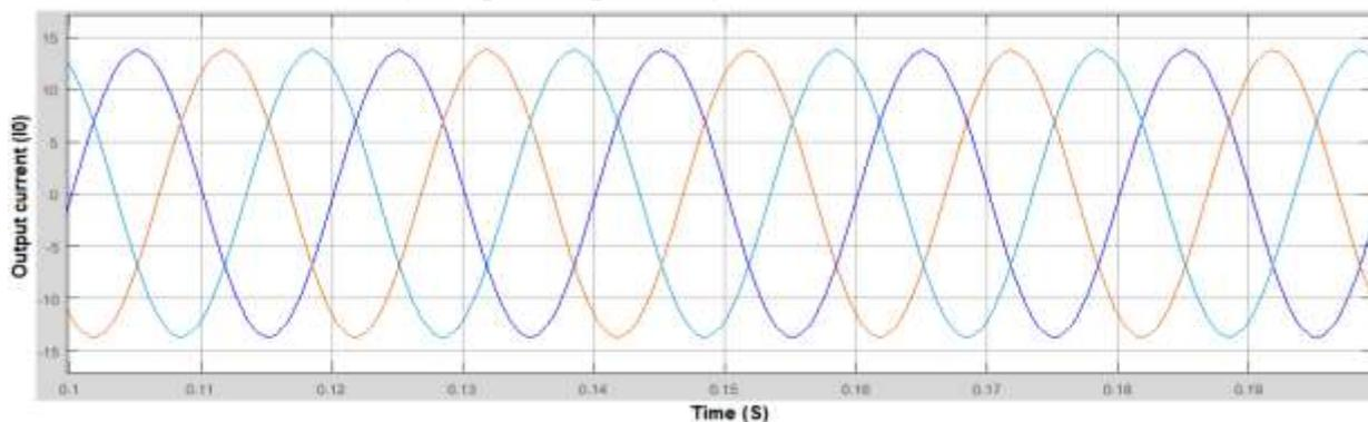
Fig.10. 3 phase output current of matrix converter
