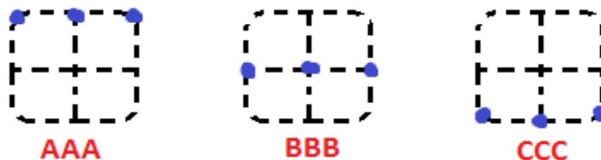
Fig.4. Matrix converter – zero vector modes
