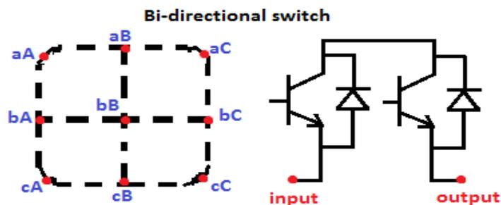
Fig.3. Matrix converter with bi-directional switch
