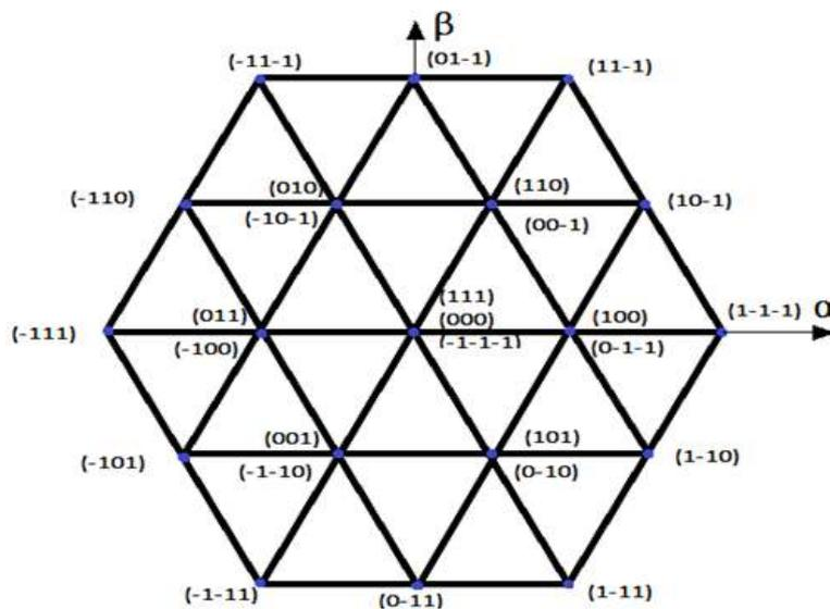
Fig.6a. Space vector representation for 3-phase power converters
