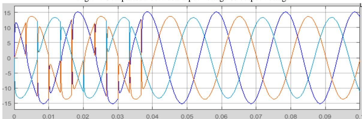
Fig.15. input current of matrix converter with 3-phase IM drive
