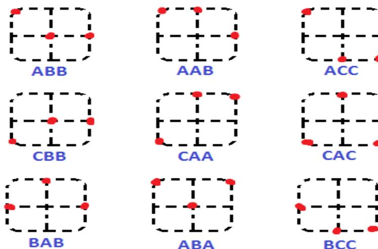
Fig.5. Matrix converter – active vector modes
