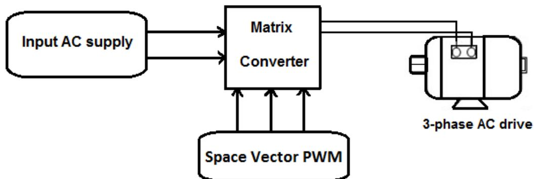
Fig.1. Block diagram of 3-phase matrix converter fed IM drive
