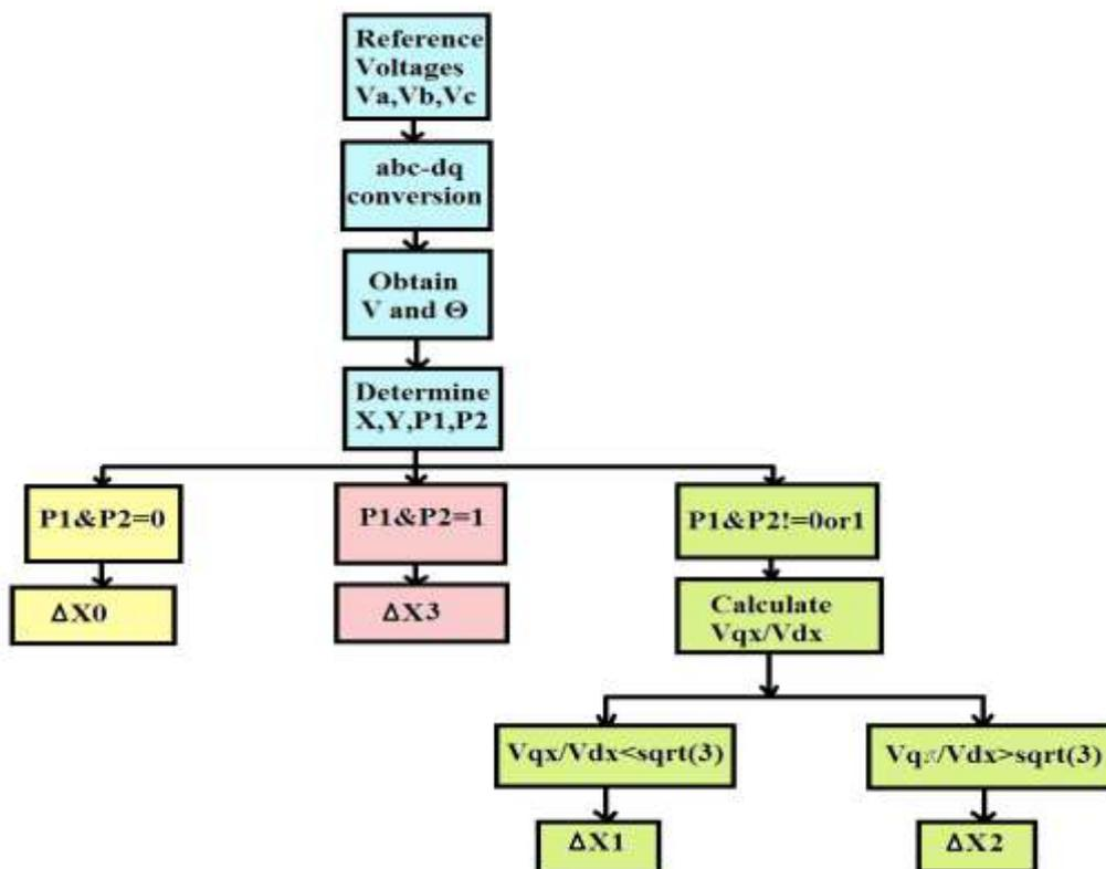
Fig.6b. Flowchart for switching pulse generation using SVPWM method
