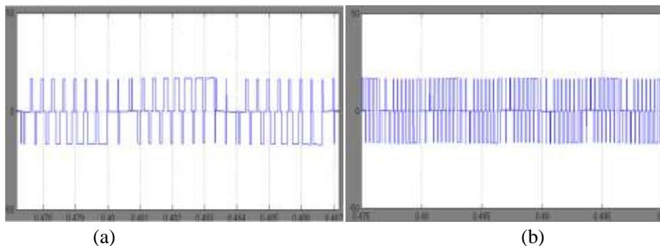
Fig.17. Common mode voltage reduction (a) a-phase (b) b-phase
