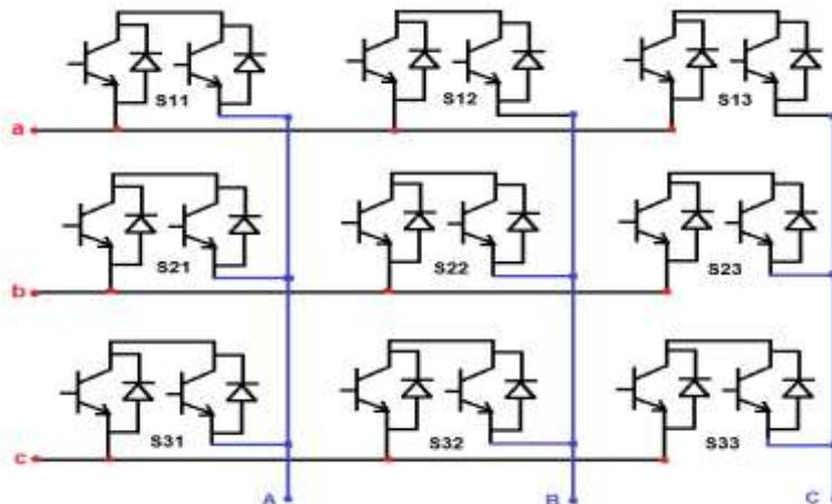
Fig.2. three-phase matrix converter
