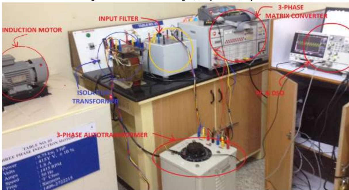
Fig.27. Experimental setup for 3-phase matrix converter with IM drive
