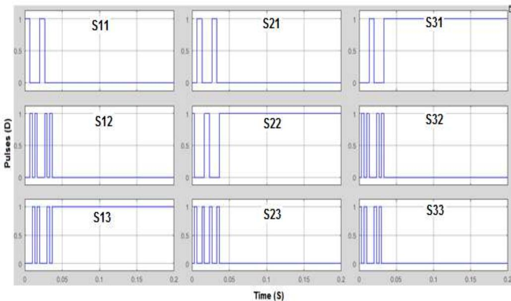
Fig.13. Switching pulse generation for matrix converter using SVPWM
