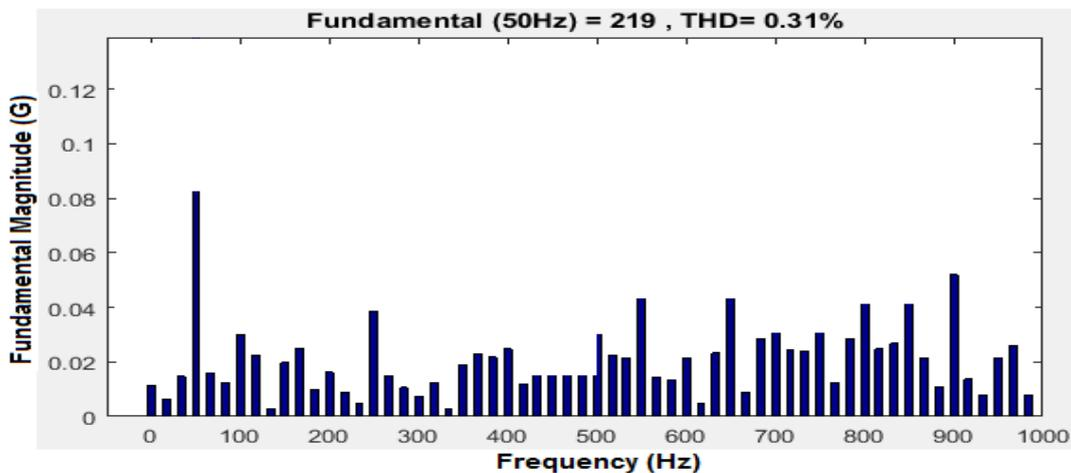
Fig.11. THD analysis for 3-phase matrix converter variable output voltage
