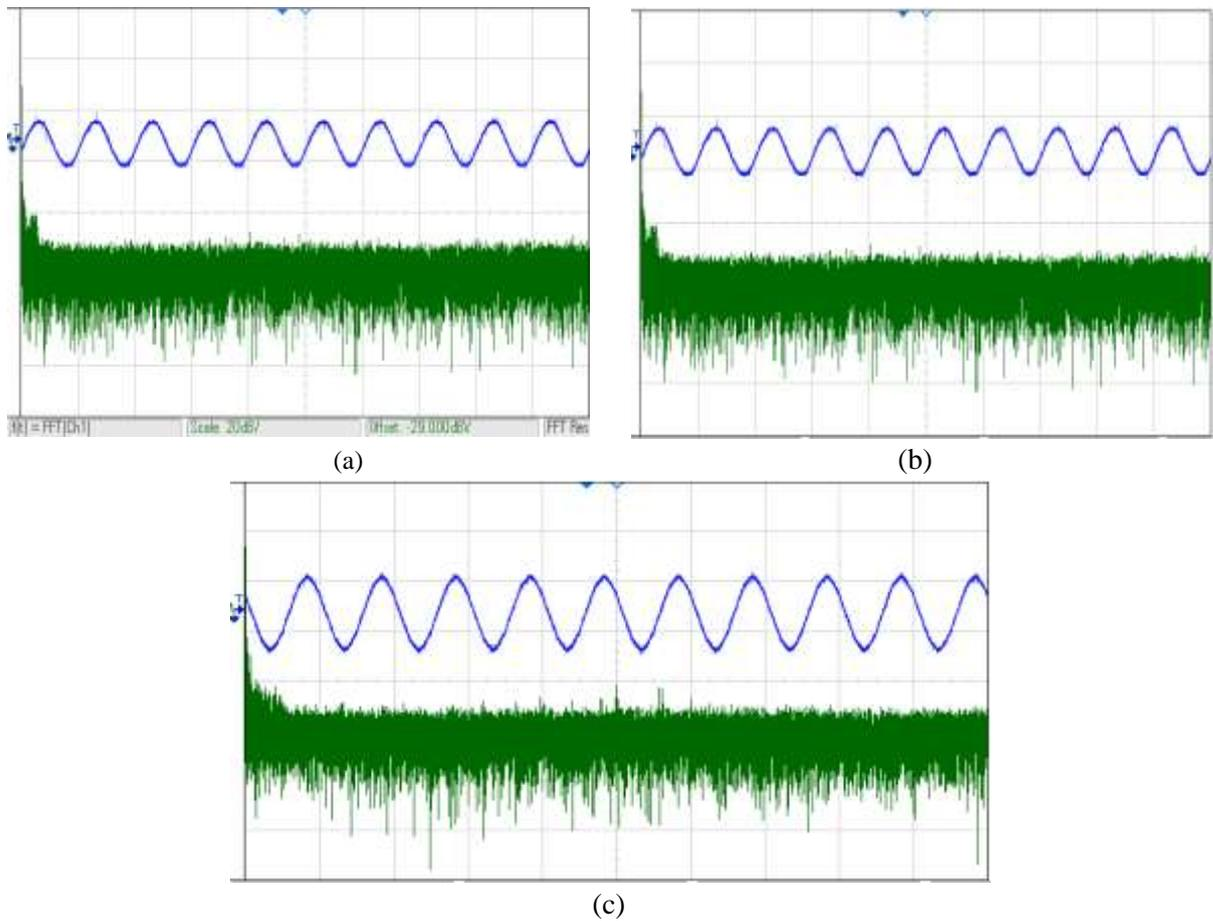
Fig.22. Output current of 3-phase matrix converter with FFT analysis (a) Ia (b) Ib (c) Ic
