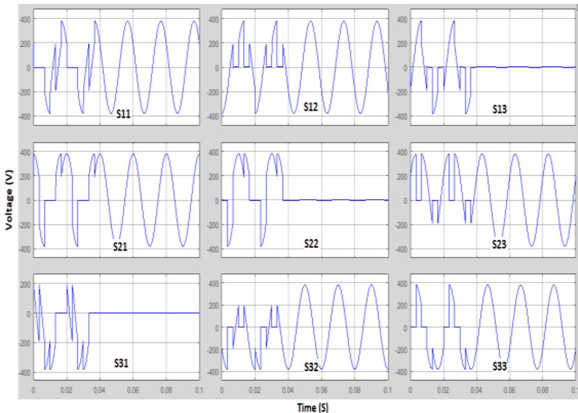
Fig.16. Voltage stress across bi-directional switches (S11, S12, S13, S21, S22, S23, S31, S32, S33)
