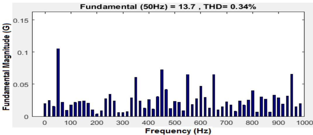
Fig.12. THD analysis for 3-phase matrix converter output current
