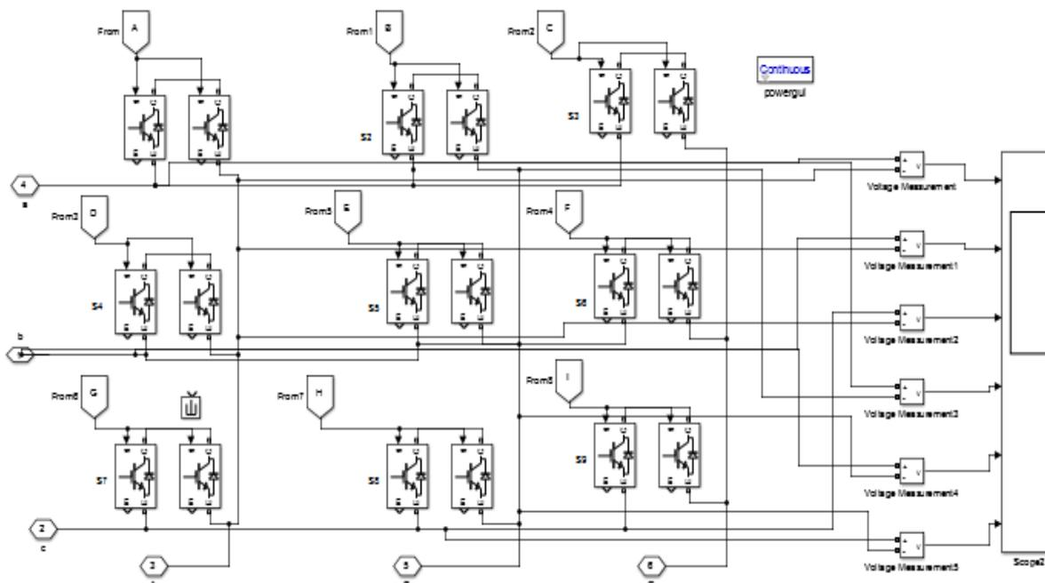
Fig.7. Simulation diagram of matrix converter
