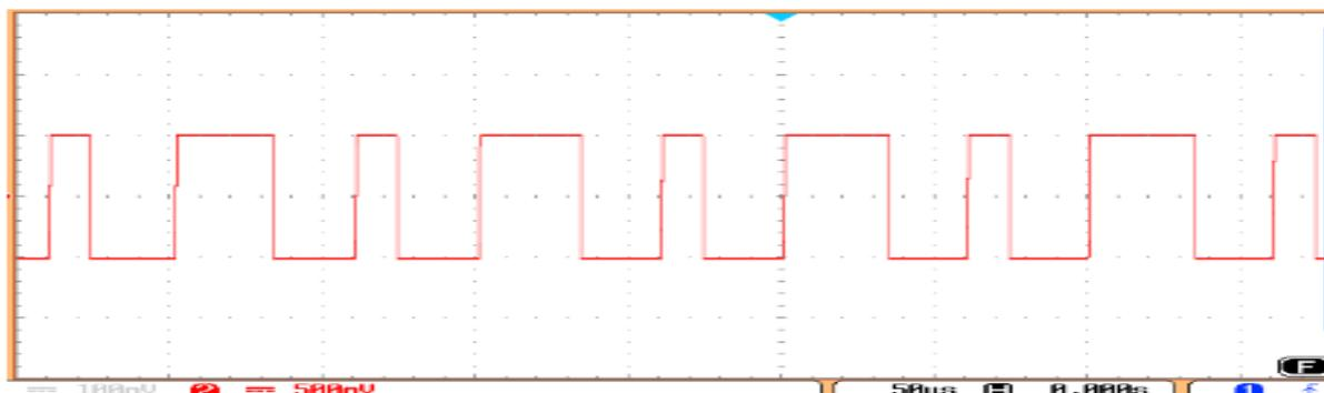
Fig.20. Gating pulse of switch S21
