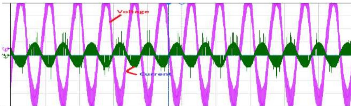
Fig.25. Output voltage & current waveform of 3-phase Matrix converter
