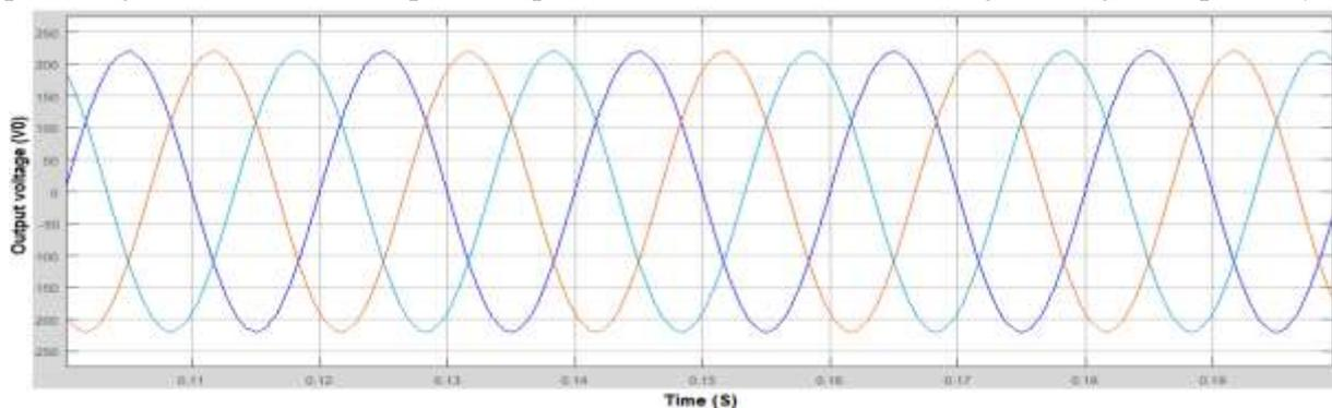
Fig.8. 3 phase variable output voltage of matrix converter
