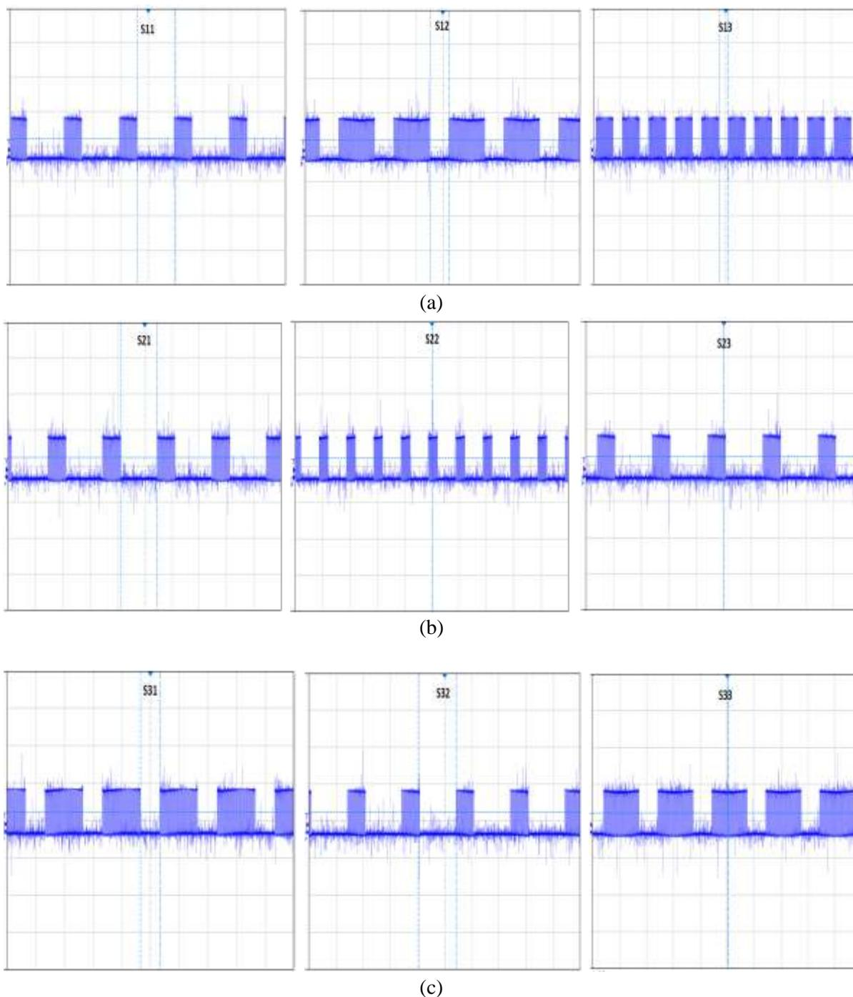
Fig.19. Gating pulses for 3-phase matrix converter (a) S11, S12, S13 (b) S21, S22, S23 (c) S31, S32, S33
