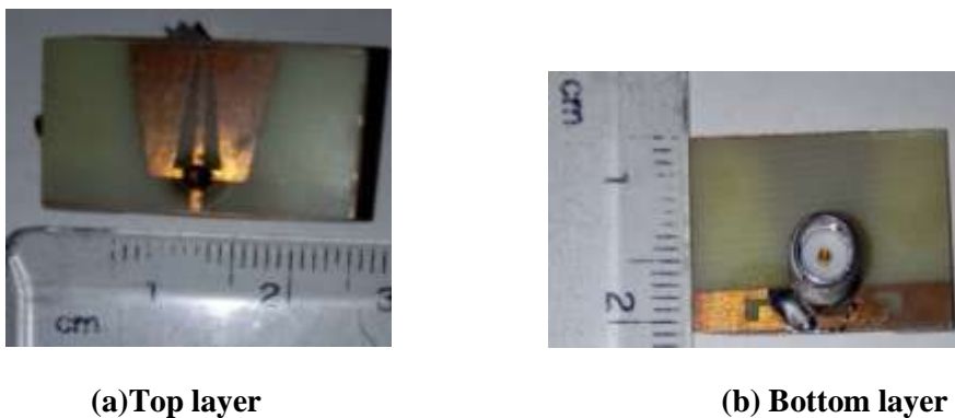
Figure 2. Fabricated geometry of the proposed antenna
