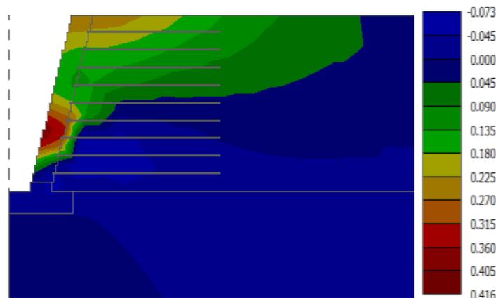
**Figure. 2.** Horizontal wall movement for soil-1, L= 2.8 m
