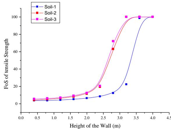
Figure. 10. Comparison of Factor of Safeties against tensile strength for three different soils
