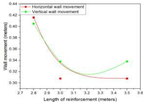
Figure. 4. Horizontal and Vertical wall movement for soil type-1
