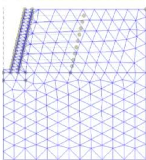
Figure. 1. Discretized MSE wall (Meshing)
