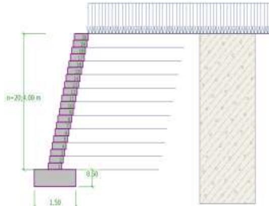
Figure. 7. MSE Wall Geometry
