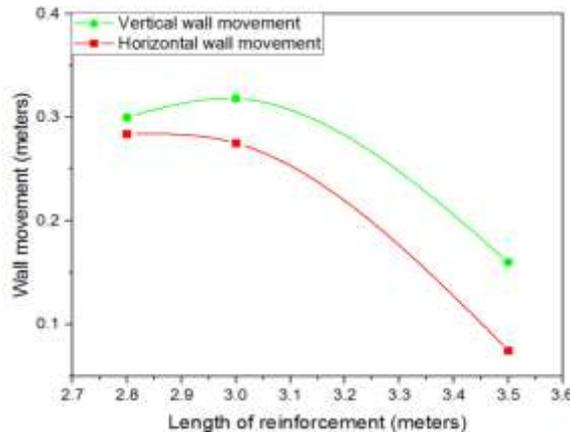
Figure. 5. Horizontal and Vertical wall movement for soil type-2
