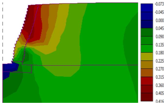
Figure. 3. Vertical wall movement for soil -1, L= 2.8 m
