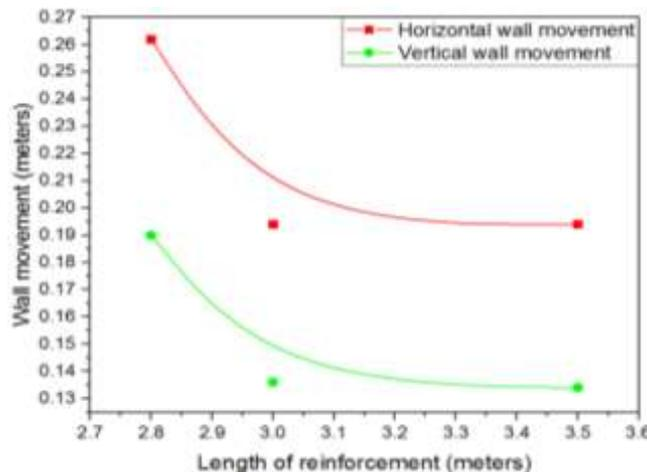
Figure. 6. Horizontal and Vertical wall movement for soil type-3
