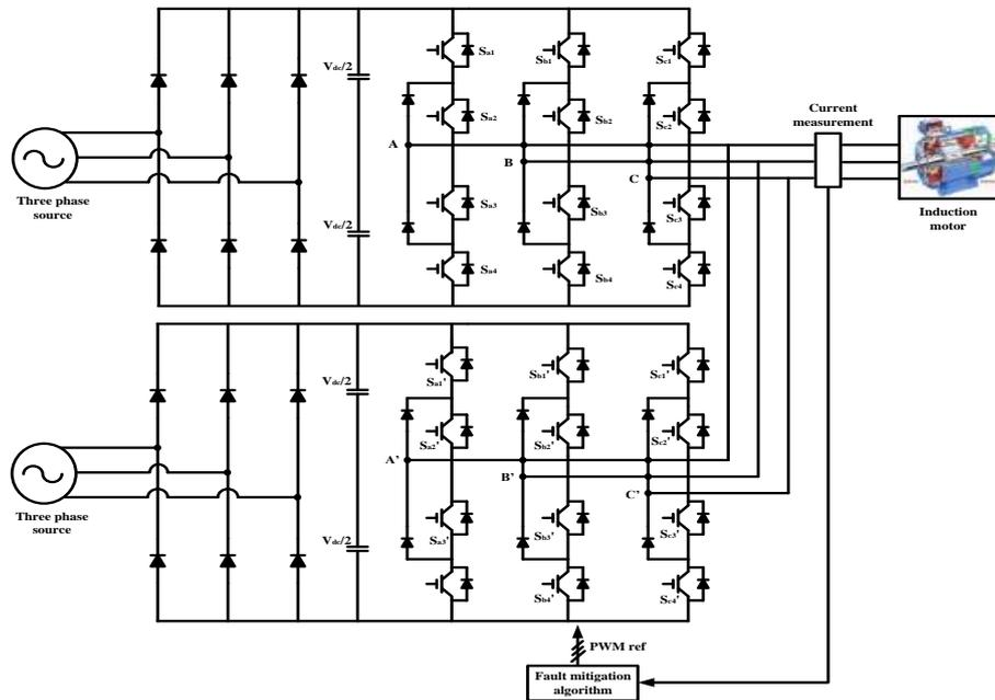
Fig.7 Parallel Diode Clamped Inverter with Fault Mitigation Algorithm
