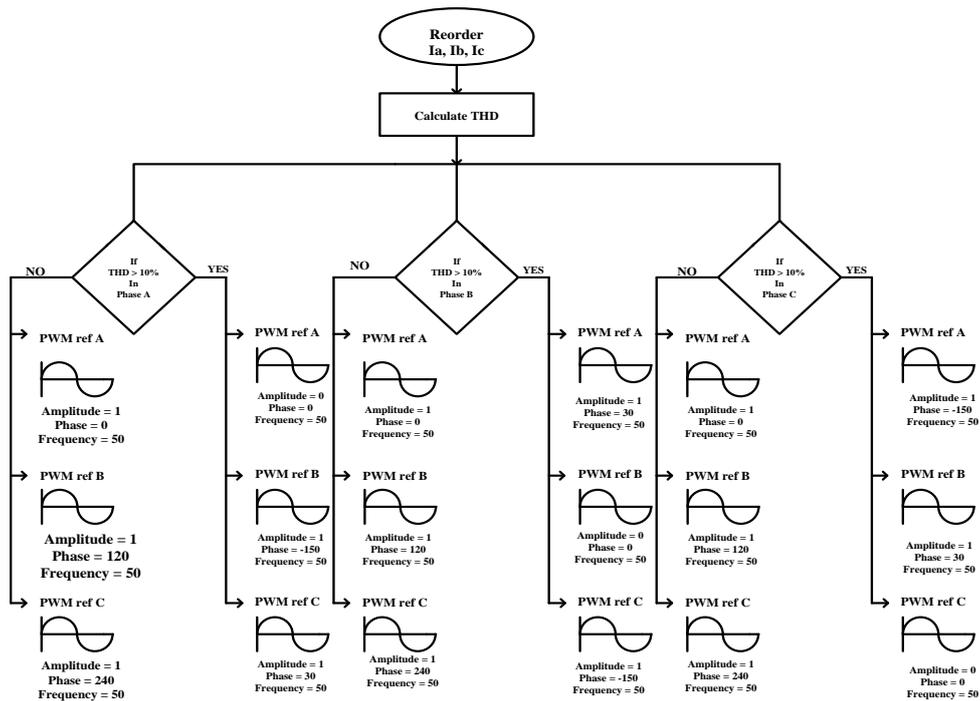
Fig.6 Fault Mitigation Algorithm
