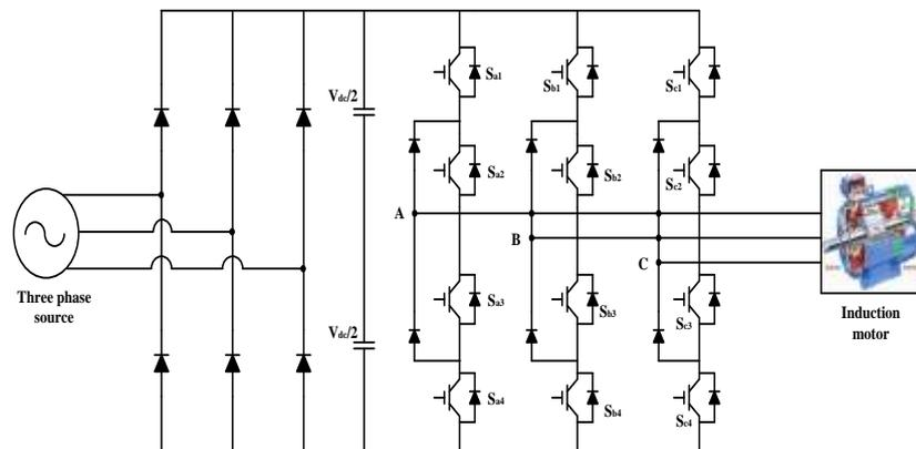
Fig.1 Conventional Diode Clamped Inverter Fed Induction Motor
