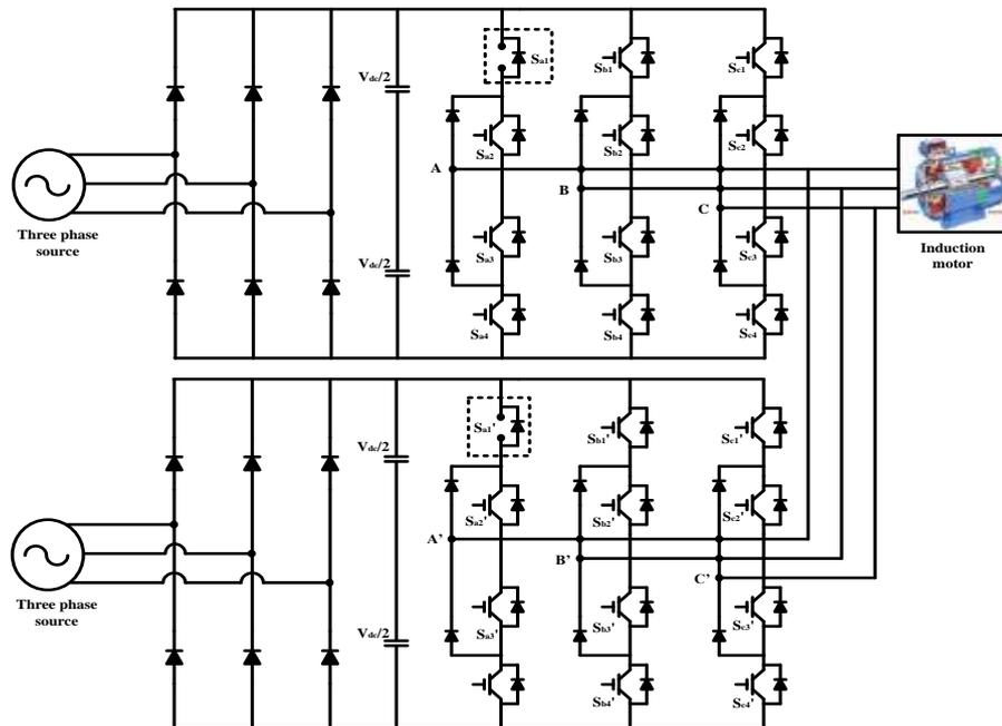
Fig.5 Fault in both parallel diode clamped inverters
