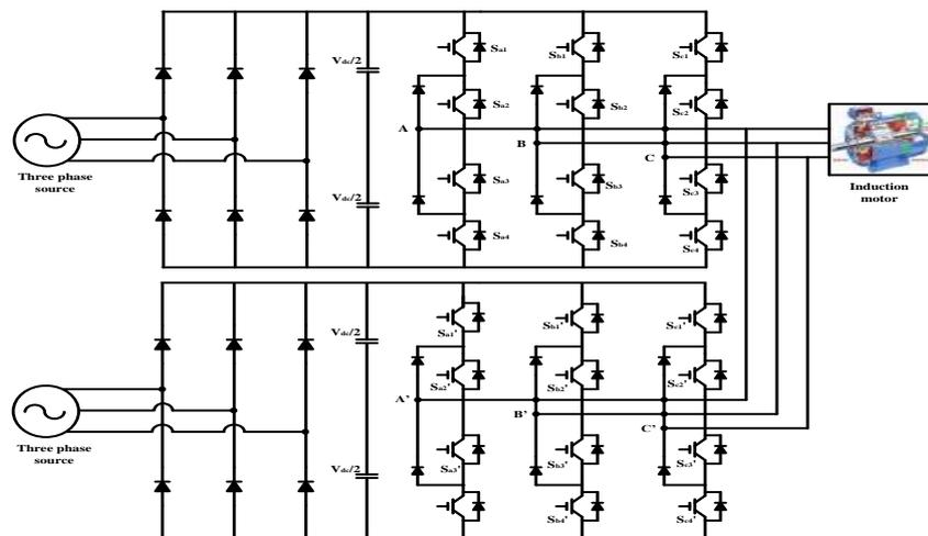
Fig.2 Two Parallel Inverter Topology Fed Induction Motor
