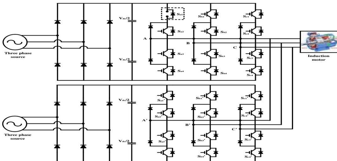
Fig.3 Fault in Upper Inverter of Two Parallel Diode Clamped Inverter Topology
