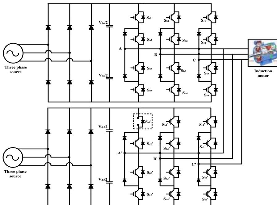
Fig.4 Fault in lower inverter of two parallel diode clamped inverter topology
