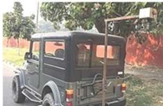
**Figure. 4.** Camera setup for recording road surface videos
