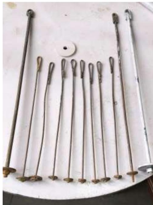
**Fig. 7: Piles used in laboratory Tests**
