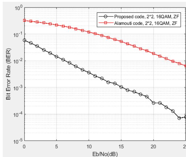
**Figure. 8.** BER Performance of proposed STBC and Alamouti codes with 16QAM modulation for ZF equalization
