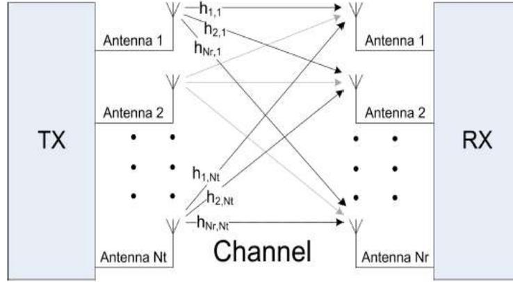
**Figure. 1.** Multiple-Input Multiple-Output system block diagram
