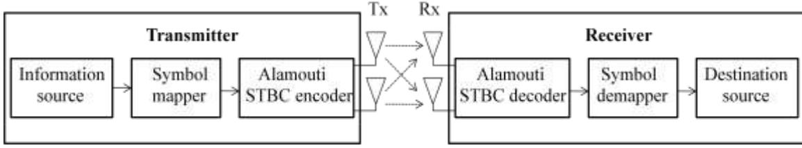
**Figure 2.** Block diagram of the Alamouti STBC-MIMO 2x2 system
