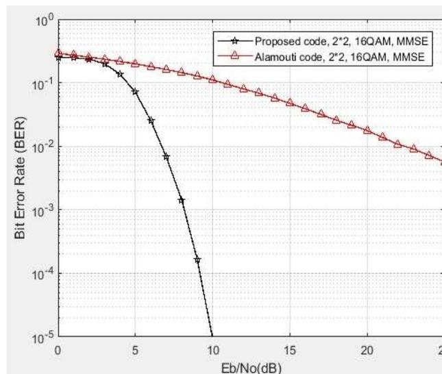
**Figure. 9.** BER Performance of proposed STBC and Alamouti codes with 16QAM modulation for MMSE equalization
