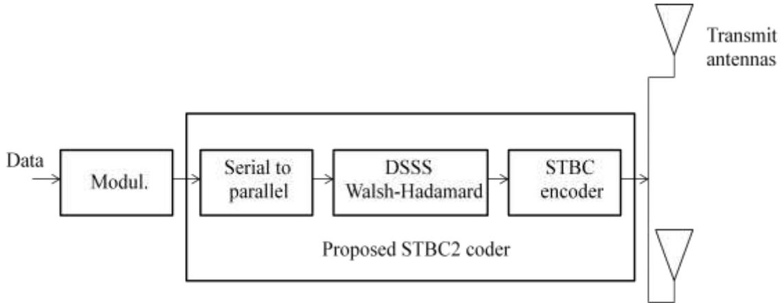
**Figure 3.** Block diagram of the proposed STBC-MIMO 2×2 system in transmission
