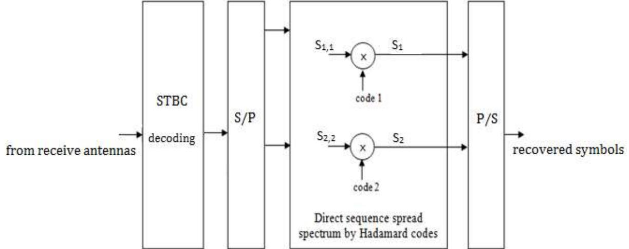
**Figure 7.** Principle of the proposed STBC2 decoding
