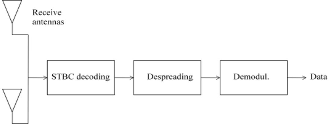
**Figure. 6.** Block diagram of the proposed STBC-MIMO 2×2 system in reception
