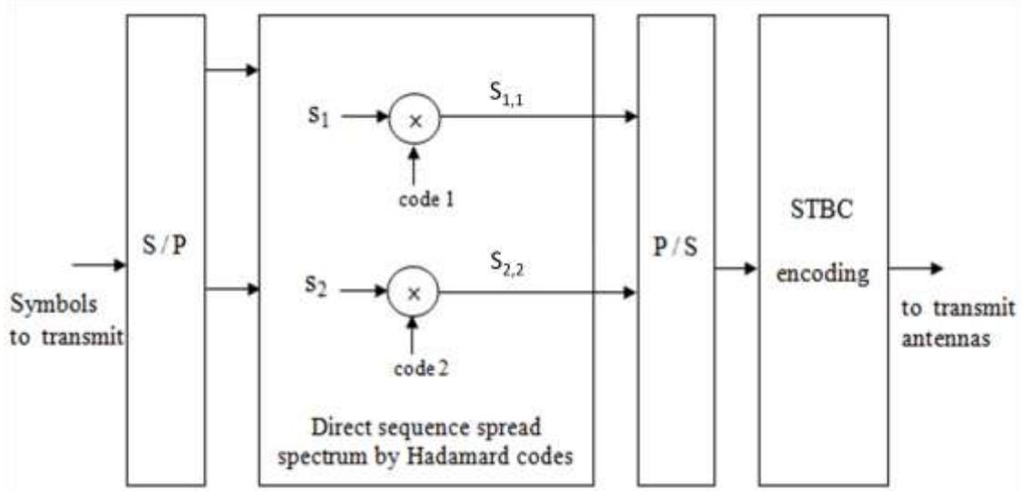
**Figure 4.** Principle of the proposed STBC2 coding
