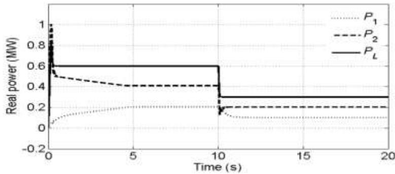
Figure 8 Load sharing among Inertial DG using Frequency droop control and Non-inertial DG using Angle droop control in Test system-B
