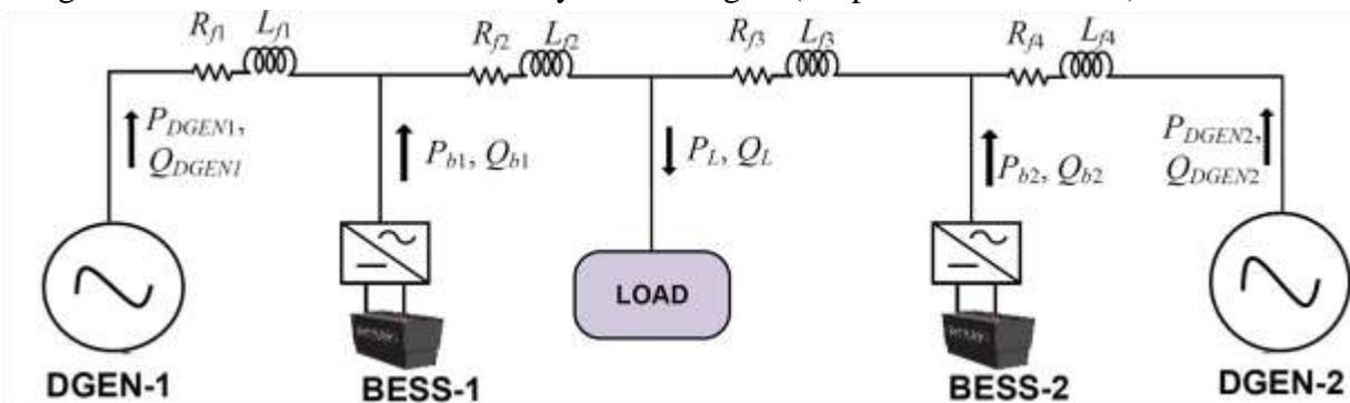
Figure 17 Structure of autonomous hybrid microgrid (Non-dispatchable DG units) with BESS
