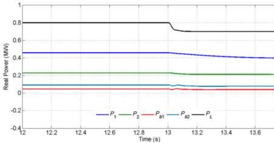
Figure 19 Real power flows of autonomous hybrid microgrid with BESS considering load variation @ 13s
