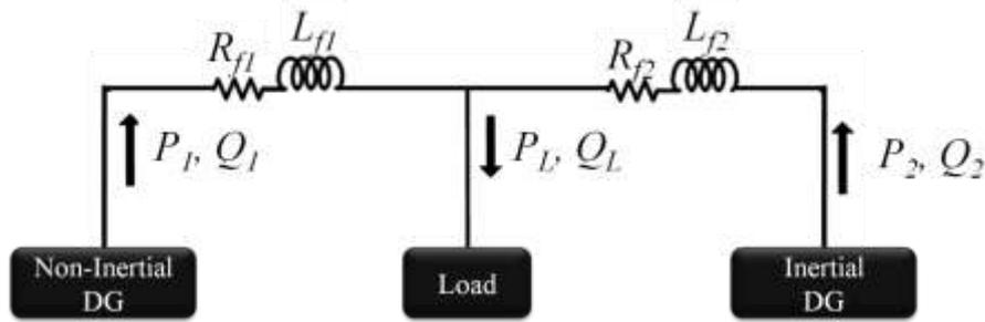
Figure 3 Block diagram of Test system-B: Autonomous hybrid microgrid with one Inertial & one Non-inertial DG units
