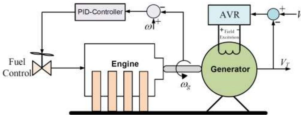
Figure 1 Schematic diagram of DGEN set- Inertial type DG unit
