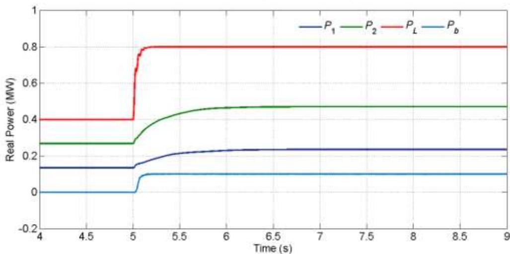
Figure 18 Real power flows of autonomous hybrid microgrid with BESS considering load variation @ 5s
