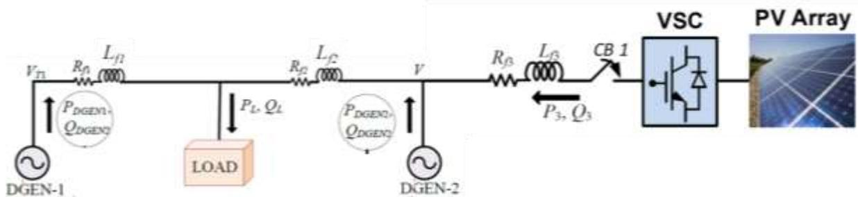
Figure 14 Schematic of PVCS integrated with microgrid Test system-A
