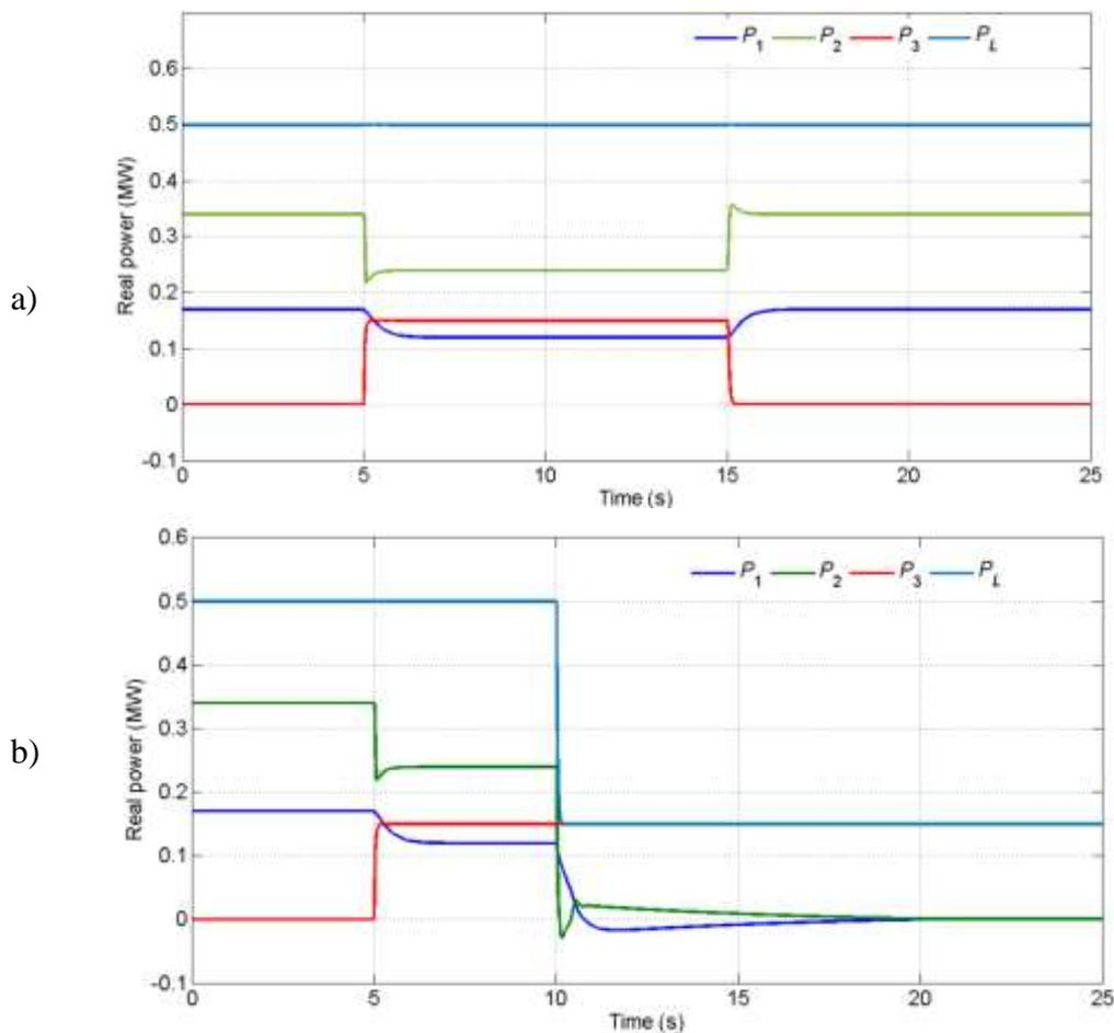
Figure 15 Real power flows in microgrid with PVCS (switched @ 5s) a) without considering load variations b) with considering load variations
