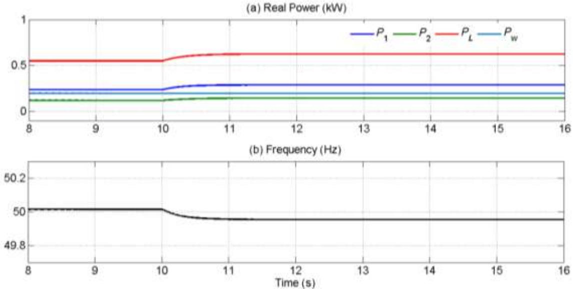
Figure 12 Real power flows in microgrid with WECS (switched @ 2s) and microgrid frequency with considering load variations
