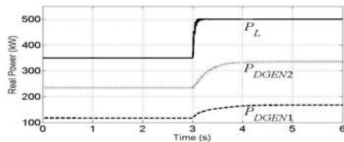
Figure 6 Load sharing among Inertial DGs using Frequency droop control in Test system-A
