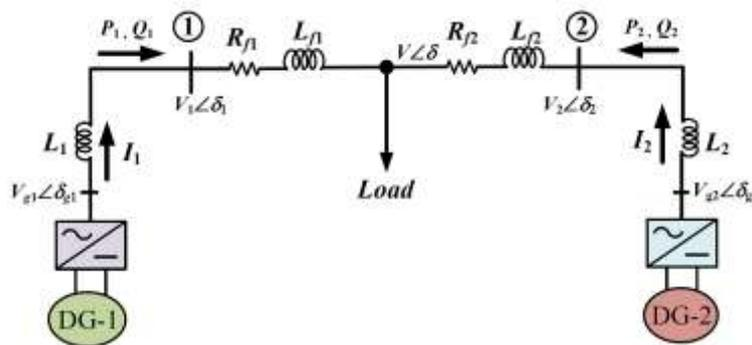
Figure 4 Block diagram of Test system-C: Autonomous hybrid microgrid with two Non-inertial DG units
