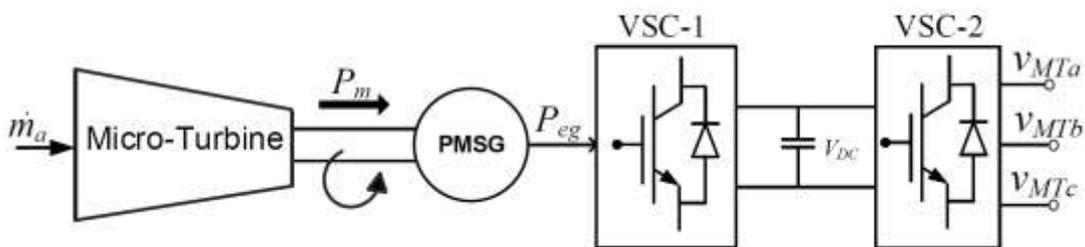
Figure 2 Schematic diagram of micro turbine with converter – Non-inertial type DG unit
