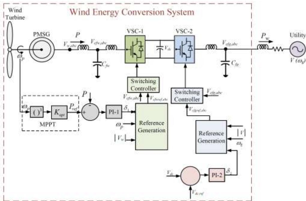
Figure 9 Schematic of WECS interconnected with utility grid
