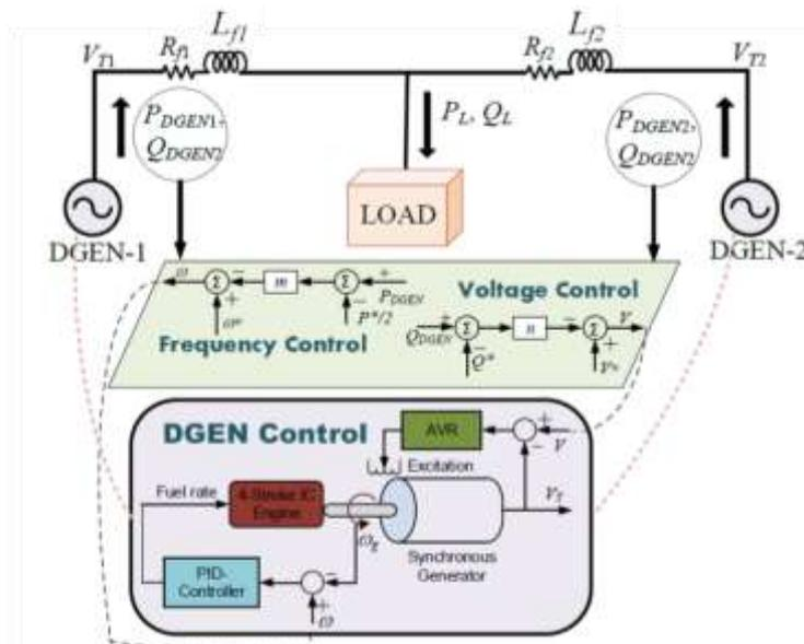
Figure 5 Block diagram of Test system-A: Autonomous hybrid microgrid with two inertial DG units
