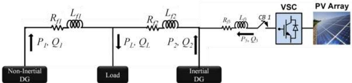
Figure 13 Schematic of PVCS integrated with microgrid Test system-B
