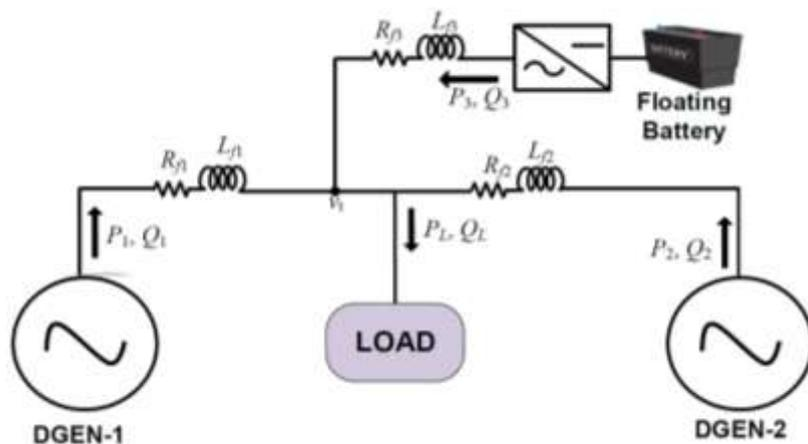
Figure 16 Structure of autonomous hybrid microgrid (Dispatchable DG units) with BESS
