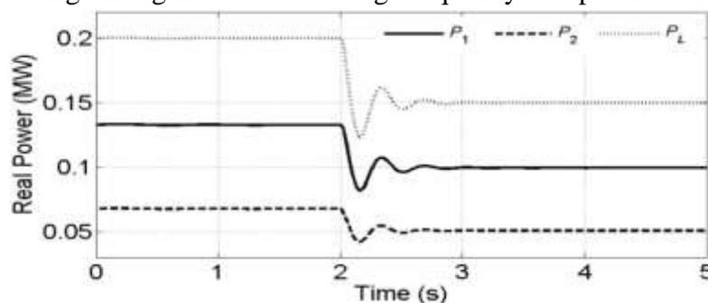
Figure 7 Load sharing among Non-inertial DGs using Angle droop control in Test system-C
