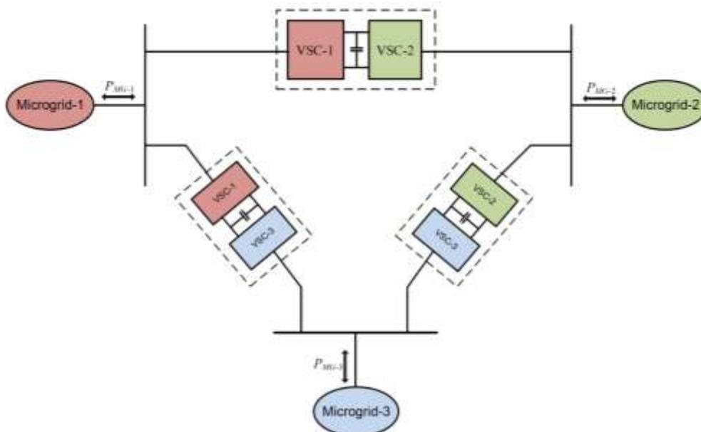
Figure 22 Three microgrids interconnected through back to back converters
