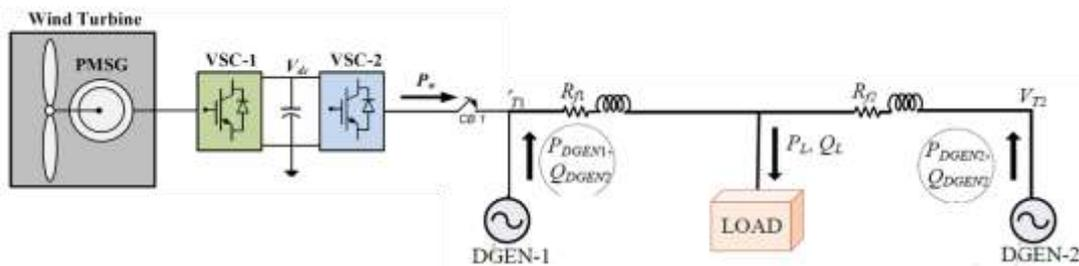
Figure 10 Schematic of WECS integrated with microgrid Test system-A
