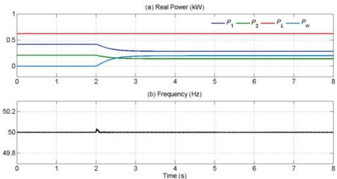
Figure 11 Real power flows in microgrid with WECS (switched @ 2s) and microgrid frequency without considering load variations
