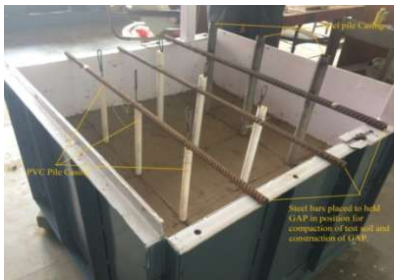
Fig. 8. Preparation of test bed and construction of GAP
