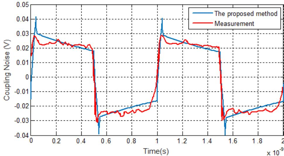
**Figure. 16.** The proposed method and measured coupling noise of TSV-Contact test vehicle (the input clock frequency at port 1 is 1 GHz)
