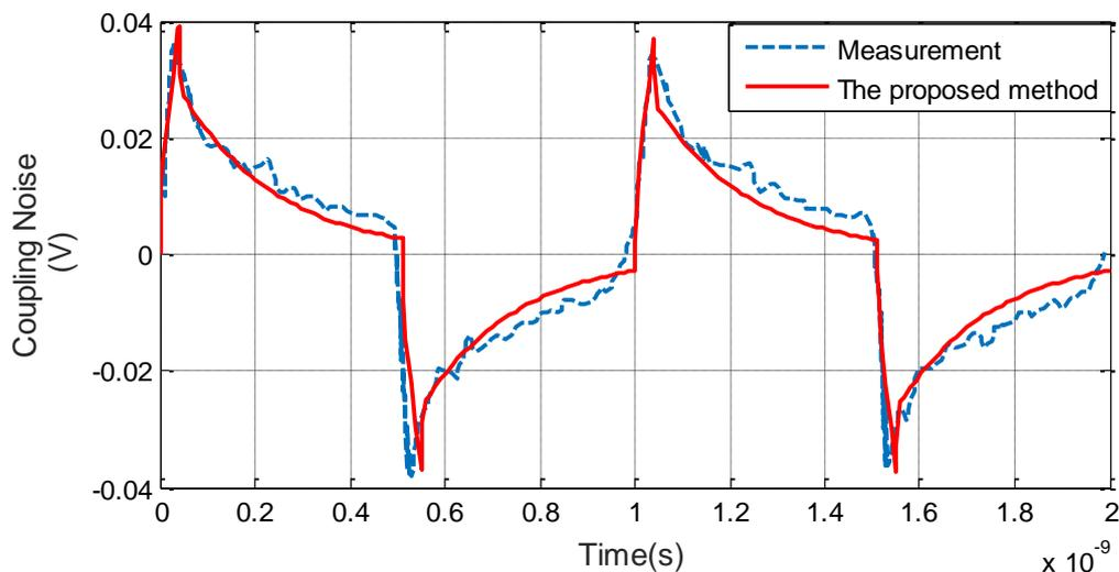
**Figure.13.** The proposed method and measured coupling of TSV-TSV test vehicle (the input clock frequency at port 1 is 1 GHz)
