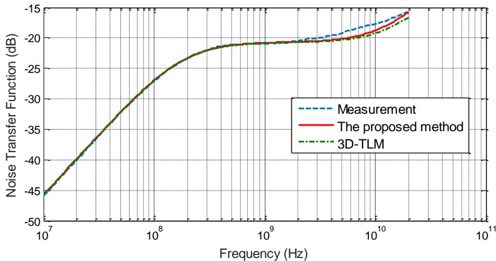
Figure 14. The proposed method, measured and 3D-TLM noise transfer function of TSV-Contact coupling
