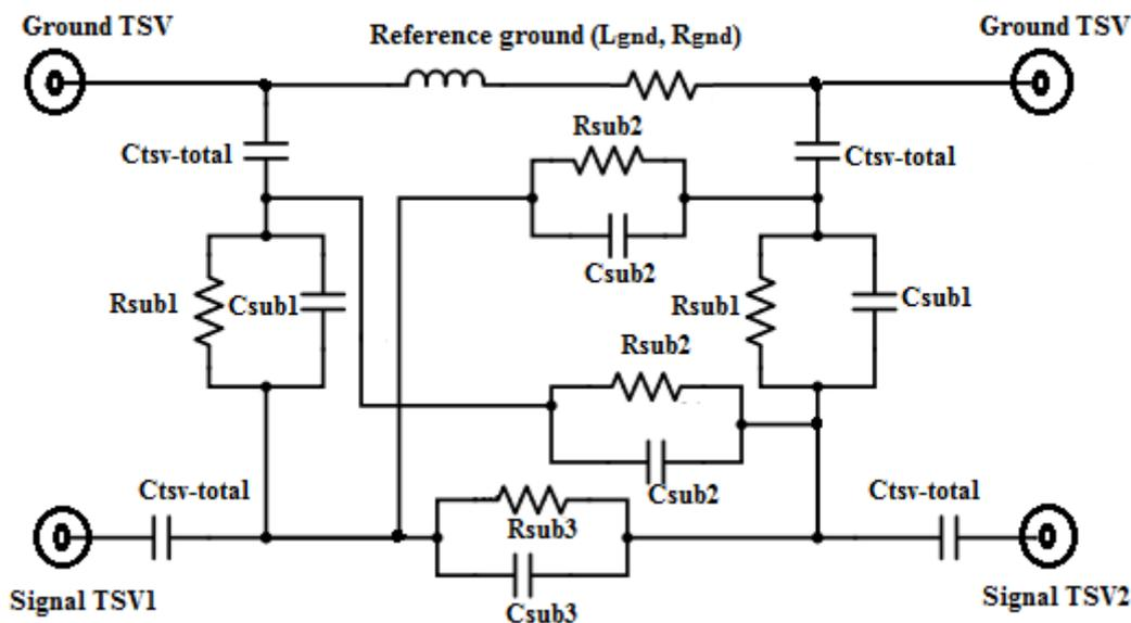
**Figure. 4.** The equivalent circuit model of TSV-TSV noise coupling
