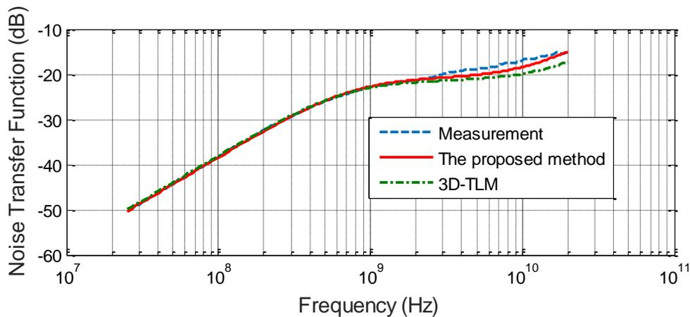
**Figure.11.** The proposed method, measured and 3D-TLM noise transfer function of TSV-TSV noise coupling
