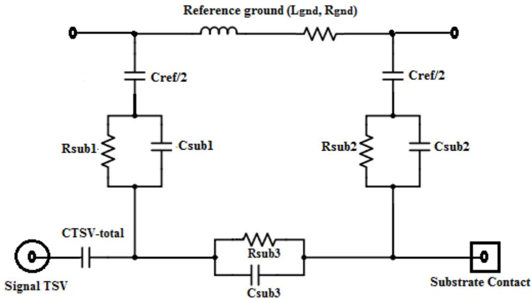
**Figure.8.** The equivalent circuit model of TSV-Active circuit noise coupling
