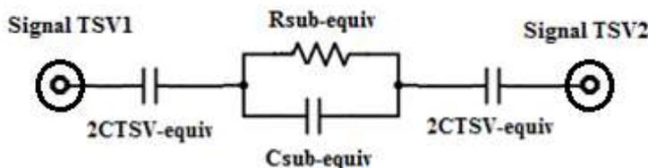
**Figure. 5.** A simplified model of the TSV-TSV noise coupling circuit
