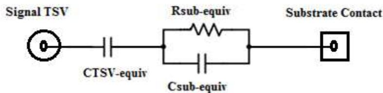
**Figure.9.** A simplified model of TSV-Active circuit noise coupling circuit
