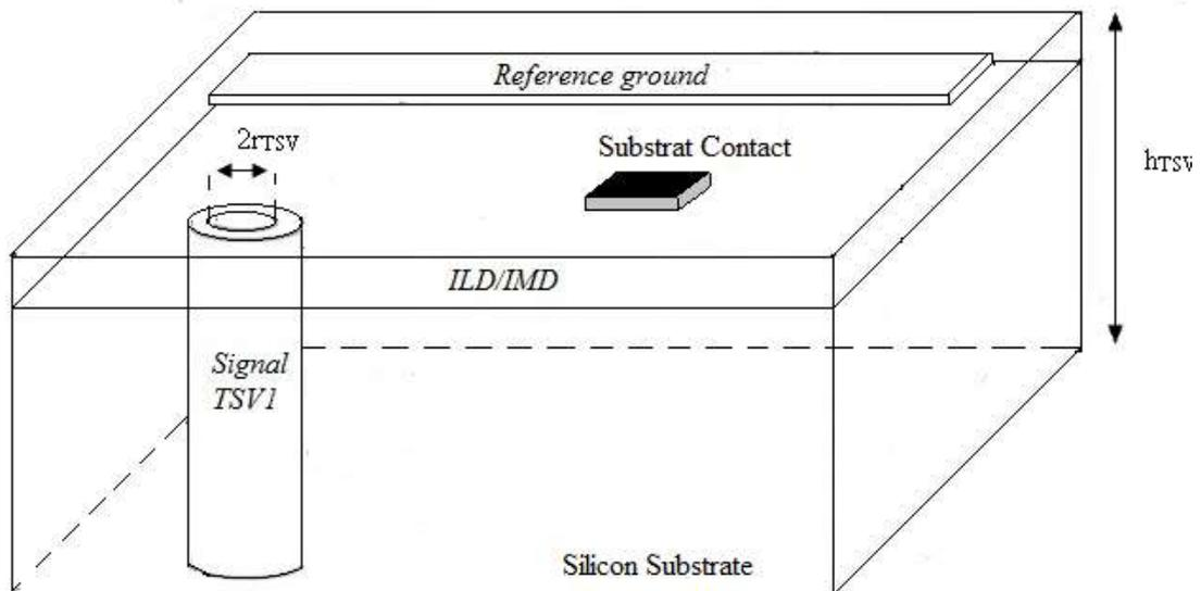
**Figure 7.** Structure of the TSV-Active circuit noise coupling
