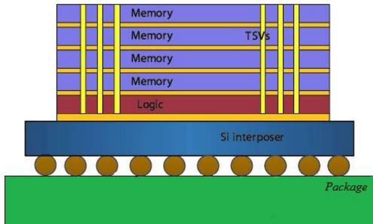
**Figure. 1.** 3D-IC using TSVs
