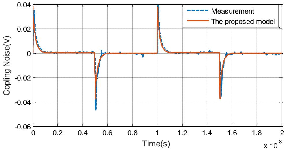
**Figure.12.** The proposed method and measured coupling of TSV-TSV test vehicle (the input clock frequency at port 1 is 100 MHz)
