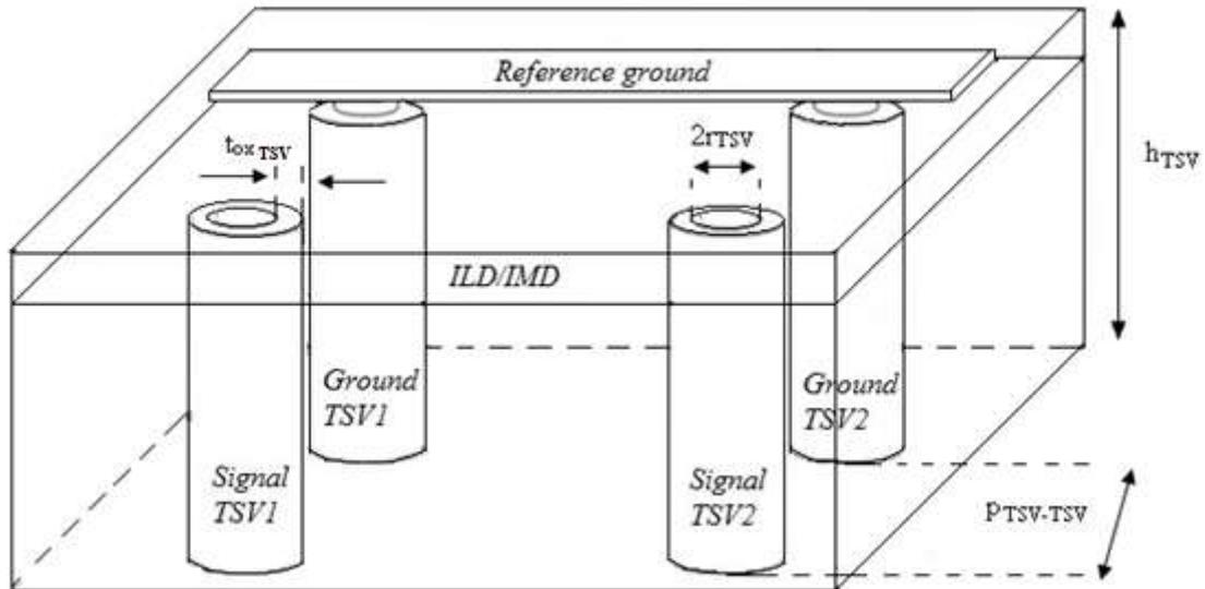
**Figure. 3.** Structure of the TSV-TSV coupling noise
