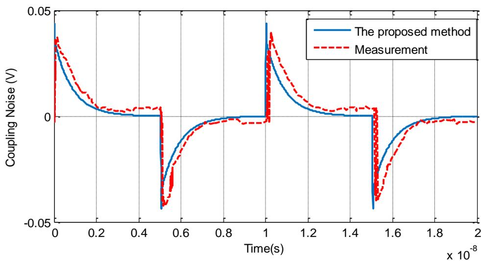
**Figure.15.** The proposed method and measured coupling noise of TSV-Contact test vehicle (the input clock frequency at port 1 is 100 Mhz)
